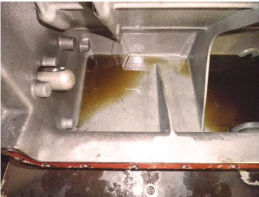
Figure 13-1: Visible chunks of metal in the sump of the disassembled engine
