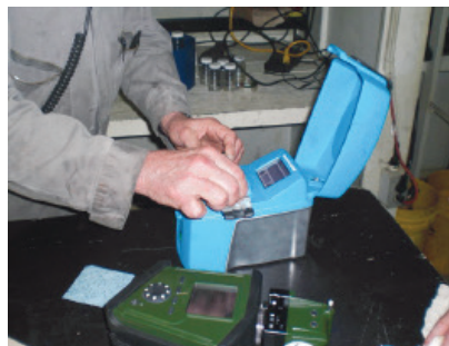
Figure 14-4: Testing air compressor oil aboard the USNS Watson, using the Q3000
