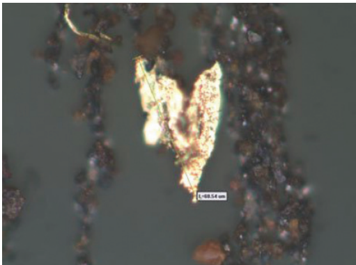
Figure 13-4: Large copper chunk seen in ferrogram image
