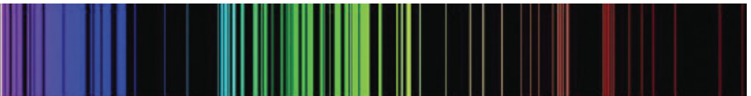
Figure 3-2: Emission Spectrum of Iron
