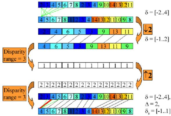
Figure 5: Overview of the hierarchical stereo calculation.
