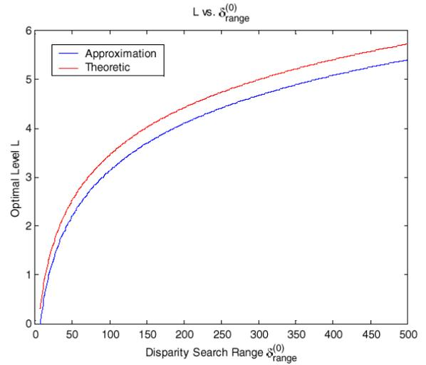
Figure 8: Interpretation of the optimal level of downsampling: approximation of the theoretic curve.
