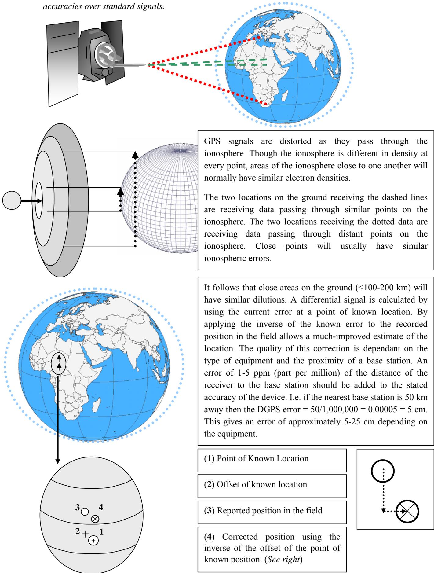
GPS signals are distorted as they pass through the ionosphere. Though the ionosphere is different in density at every point, areas of the ionosphere close to one another will normally have similar electron densities.
