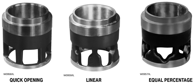
Figure 3-28. Characterized Cages for Globe-Style Valve Bodies
