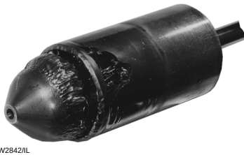
Figure 5-6. Typical Appearance of Flashing Damage
