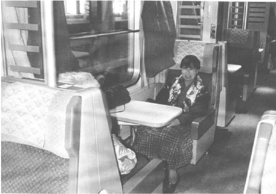
Figure 3.44 Swedish "post-modern" interior with 3+1 seating and light wooden material (class B2)
