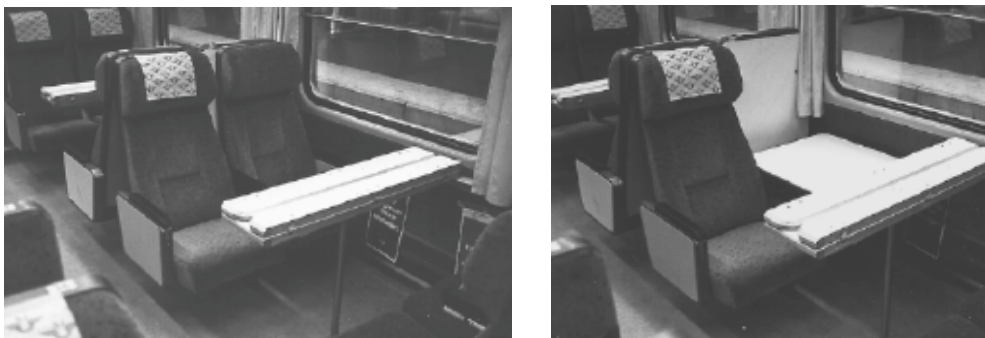
Figure 3.28 Backrest that is convertible to a "table" beside you. This particular design is used in the Swedish family cars, for parents with babies. A modified design would be needed for use in ordinary flexible purpose cars.
