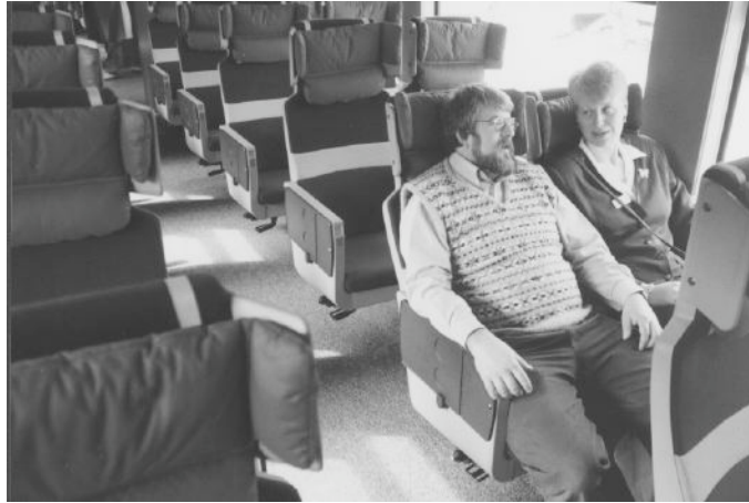
Figure 3.22 Norwegian ICE (express) train with non-facing (face-to-back) turnable seats.
