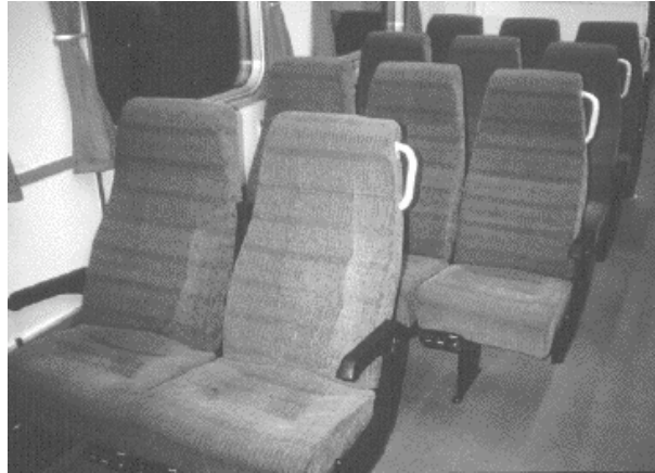
Figure 3.31 Some Swedish EMUs (X14) has 2+2 seating with 53 cm wide seats and 3+2 seating with 48 cm bus type seats. Both seat widths shown here.
