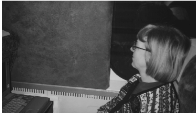
Figure 3.42 To sit by a window pillar reduces sight out of a window. About half of this passengers' view is reduced – blind spot in the drawing below.
