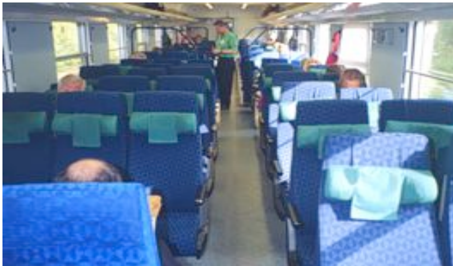
Figure 0.3 Interior of the "InterRegioMax" test coach with 2+3 seating.
