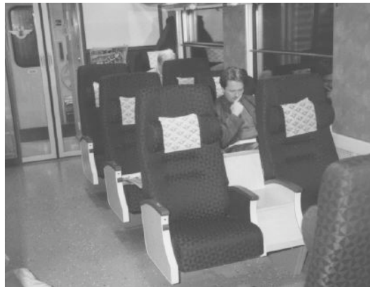
Figure 3.26 First class salon with the same seat type as in second class but separated by a "table". Swedish InterRegio coach rebuilt from InterCity 1980 coach.
