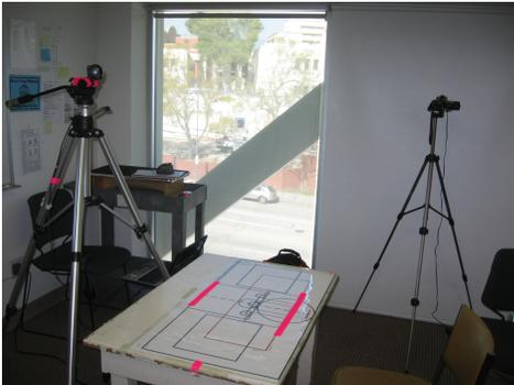
Fig. 1: Standardized WMFT setup, showing the camera positions, the testing table, and the template.
