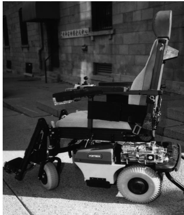
Figure 6 Autonomous wheelchair TAO-1. Cover is removed to show autonomy unit.
