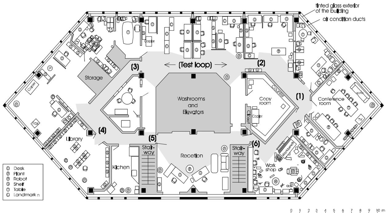
Figure 9 The office space which contains the test loop
