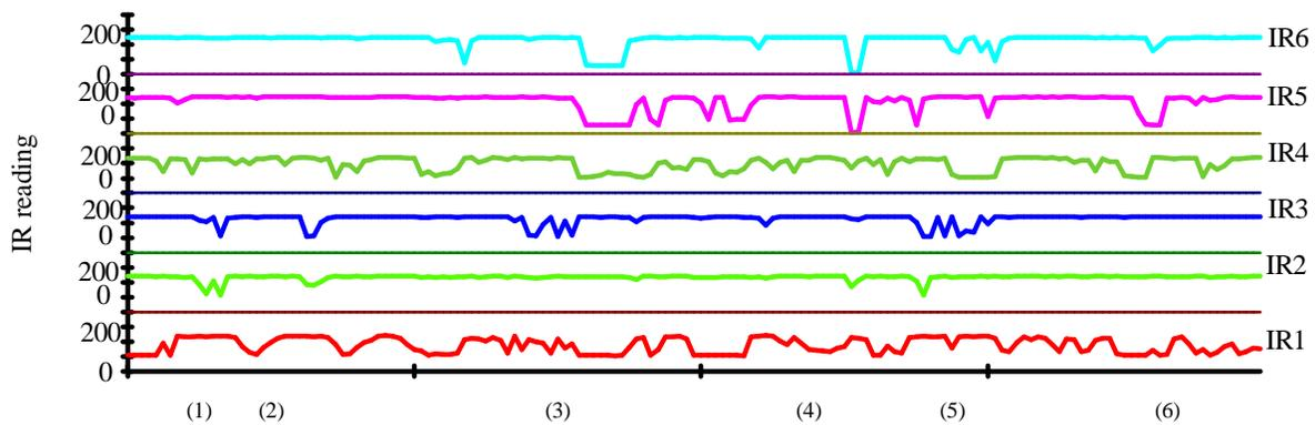
Figure 10a Output of active infrared (IR) sensors
