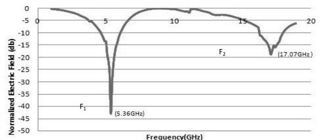
Fig 8: Normalized Transmitted Electric Field vs. Frequency for the modified Design.
