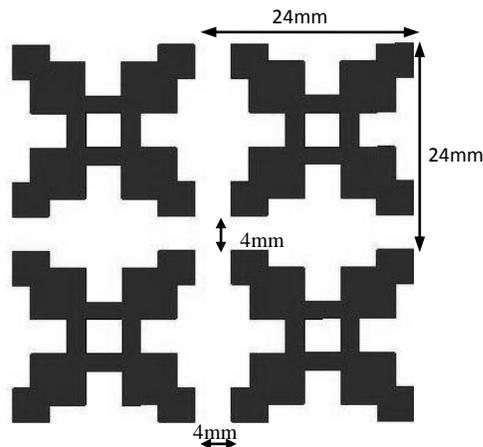
Fig2: FSS showing four unit cell and spacing between them.
