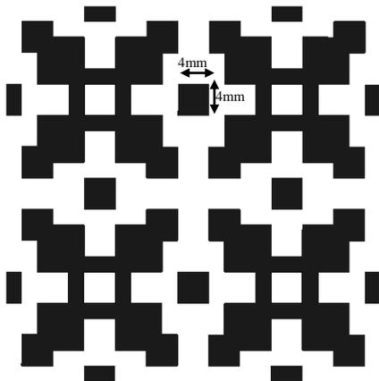
Fig4: FSS showing four unit cell with modified design.
