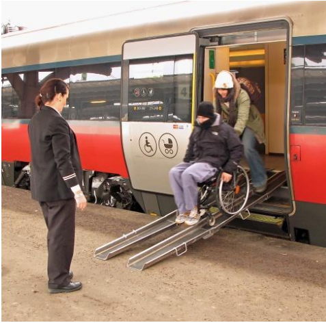
Figure 45. Manually fitted wheelchair ramps on NSB's BM73 multiple unit train. Handling a wheelchair at an intermediate station leads unfailingly to delays because of the complicated procedure.
