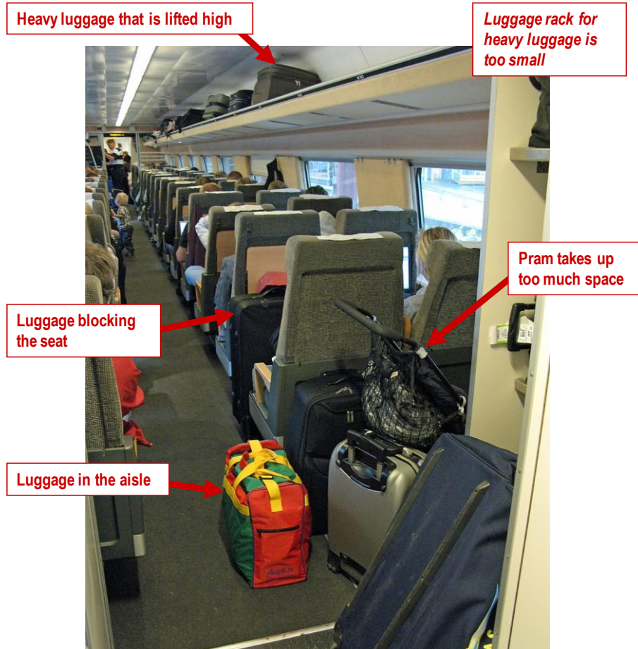
Figure 49. Examples of undesirable yet typical placing of luggage on the X 2000 as a result of insufficient luggage racks for heavy luggage. At peak loading times, travellers have even more luggage, making the problem worse.
