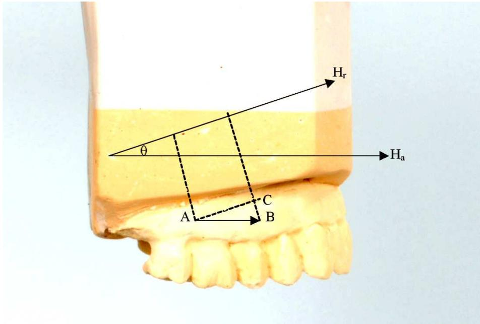
Figure 2. Model displaced by a distance AB parallel to the axis  $H_a$  parallel to the articulator cross bar produces displacements relative to the reference axes  $H_r$  and  $V_r$ .
