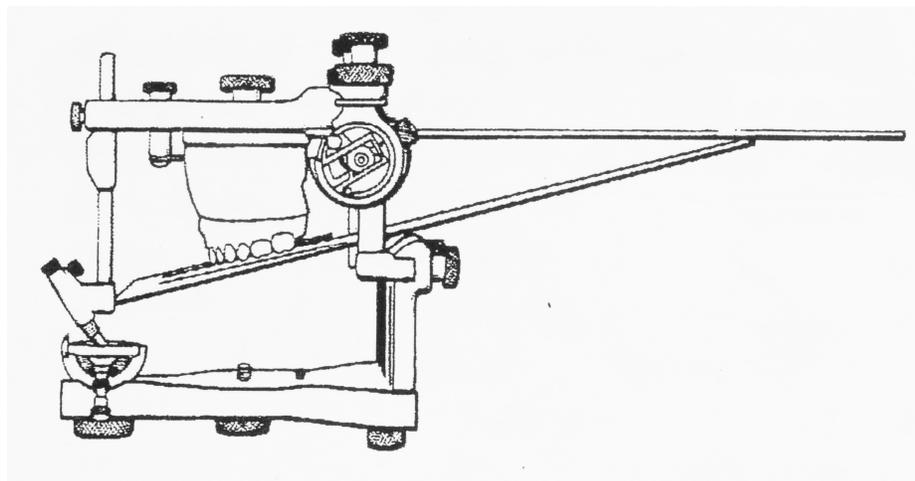
Fig.2.4. Articulator with Fox Plane modified for angle measurements.
