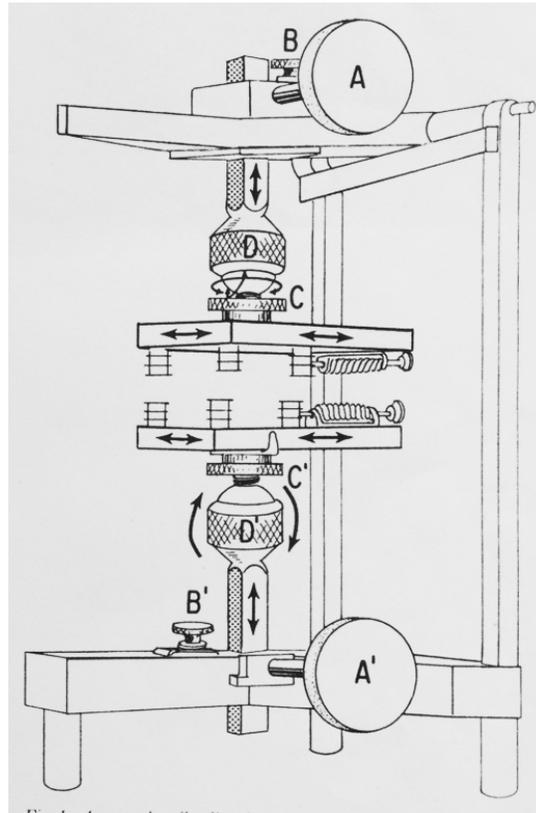
Fig.2.7. A & A' provide vertical movement. B & B' allow lateral movement. C & C' allow anterior- posterior movement and D & D' allow the casts to be rotated. Angelillo et al (1977).
