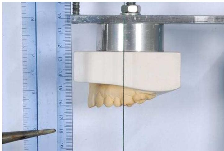
The third image was taken in the impacted position (10mm impaction incorporated) with no spacers used (Fig.4.6.).
