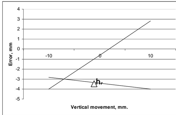
Graph 4.1. The dependence of the vertical and horizontal errors,  $\Delta v_r$  and  $\Delta h_r$ , on the vertical movement,  $v_a$ . The horizontal movement,  $h_a$ , is an advancement of 10mm.  $\theta$  is  $20^\circ$ .
