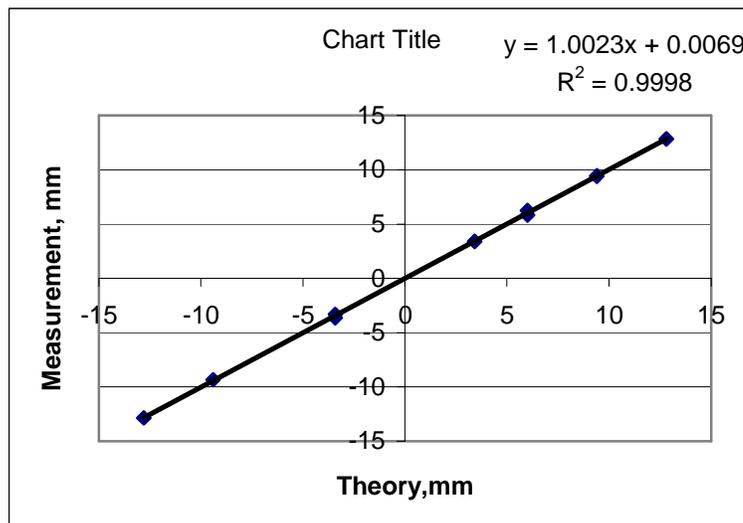
Graph 4.3: A statistical representation of the correction between the predicted theoretical values of the displacement and experimental values obtained. Data from table 4.1.
