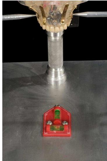
Fig.5.4. Spirit levels attached to measuring device base.
