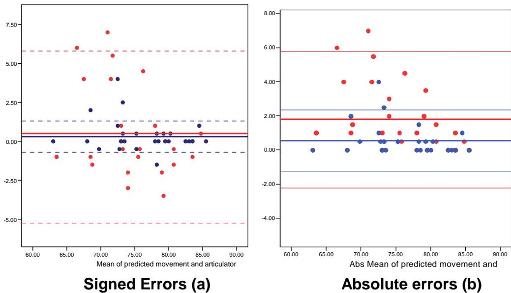
Graph 5.6a&b. Bland Altman plot showing Vertical errors (vertical axis) of **Standard** and **Orthognathic** articulators.
