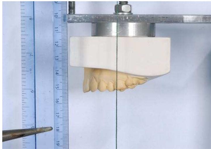
The second image was taken in the downgrafted position (10mm downgraft incorporated) using the 20mm spacer (Fig.4.5.).
