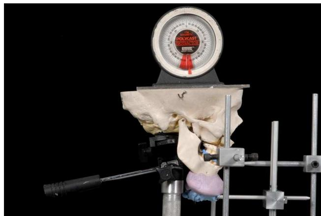
Fig.5.8. Adjusting the skull to achieve the angle required.
