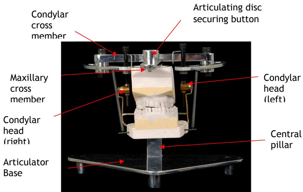
Figure.2.15. Frontal view of the maxillary and mandibular cast mounted on the Orthognathic articulator.
