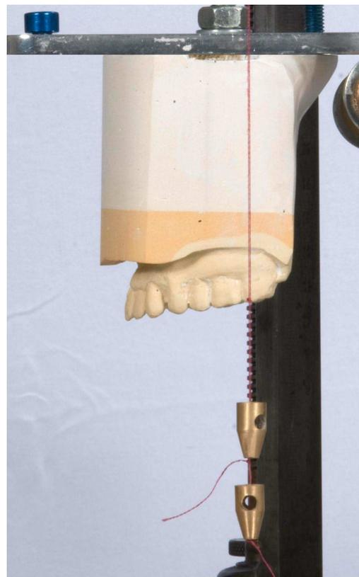
Fig.4.3. Maxillary model in initial position. Each of the two red threads supports a brass bob.
