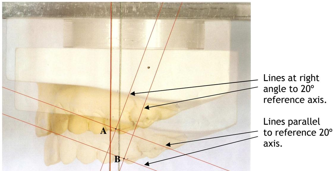
Fig.4.7. Superimposed images of model in initial and displaced positions. Vertical and parallel lines pass through the black reference mark on the model in the displaced (A) and initial (B) position.
