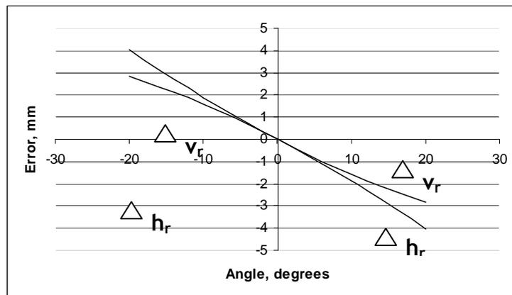
Graph 4.2. The dependence of the vertical and horizontal errors,  $\Delta v_r$  and  $\Delta h_r$ , on  $\theta$ . The horizontal movement,  $h_a$ , is an advancement of 10 mm and the vertical movement,  $v_a$ , is a downgraft of 10 mm.
