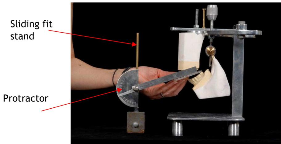
Fig.5.20. Protractor on a sliding fit stand measuring the maxillary occlusal plane angle.
