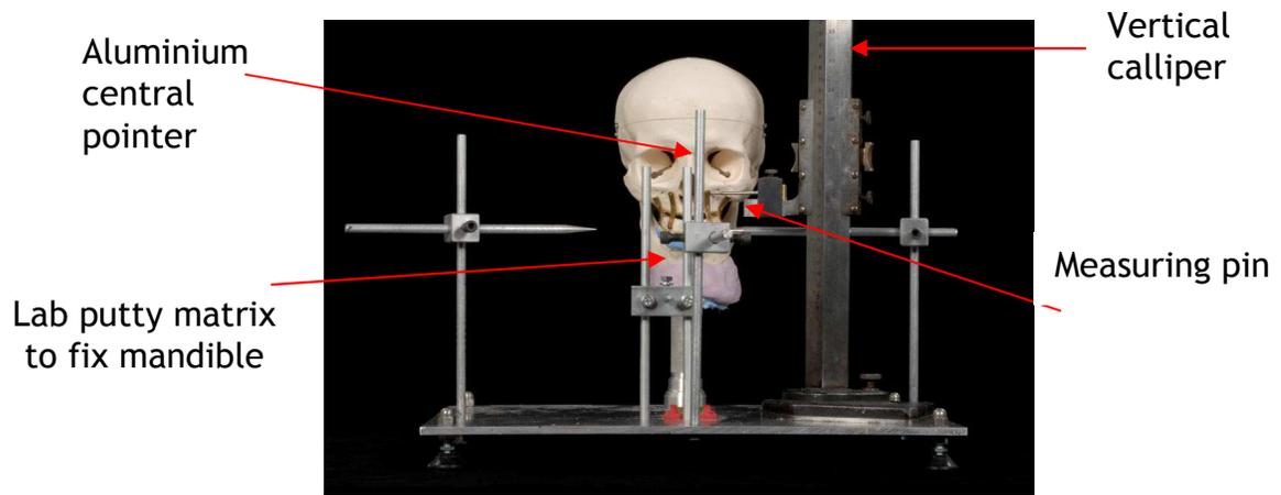
Fig.5.19. Plastic skull set in a predetermined angle with the vertical calliper for measurements.
