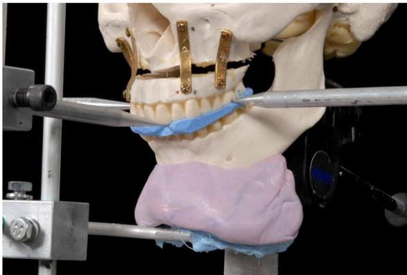
Fig. 5.2. Brass plates with cortical titanium screws fixing the maxilla in place.
