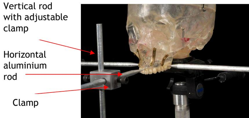
Fig. 5.18. Aluminium rod attached horizontally by a clamp.
