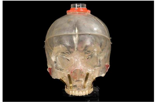
Fig.5.9.a&b. Circular spirit level secured to top of skull.
