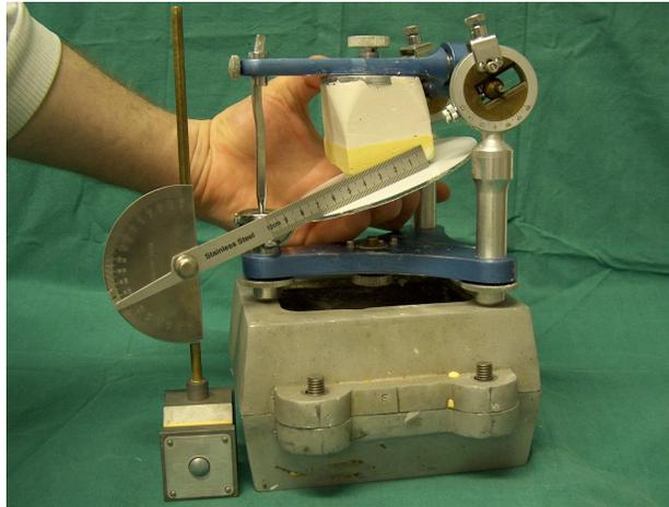
Fig.2.14. Protractor on a slide fit stand to measure the maxillary occlusal plane angle. Walker (2008a).
