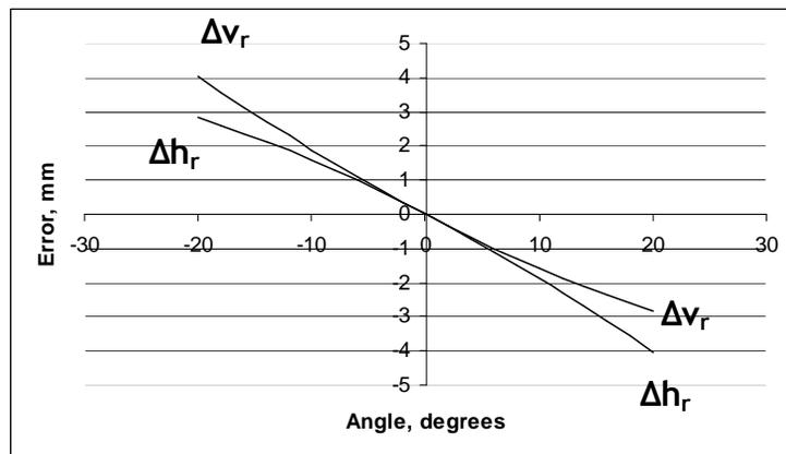
Graph 4.2. The dependence of the vertical and horizontal errors,  $\Delta v_r$  and  $\Delta h_r$ , on  $\theta$ . The horizontal movement,  $h_a$ , was an advancement of 10 mm and the vertical movement,  $v_a$ , was a downgraft of 10 mm.
