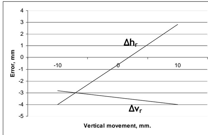
Graph 4.1. The dependence of the vertical and horizontal errors,  $\Delta v_r$  and  $\Delta h_r$ , on the vertical movement,  $v_a$ . The horizontal movement,  $h_a$ , was an advancement of 10mm.  $\theta$  is  $20^\circ$ .
