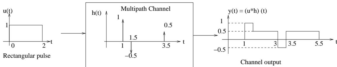
Figure 2.14: A rectangular pulse through a multipath channel.
