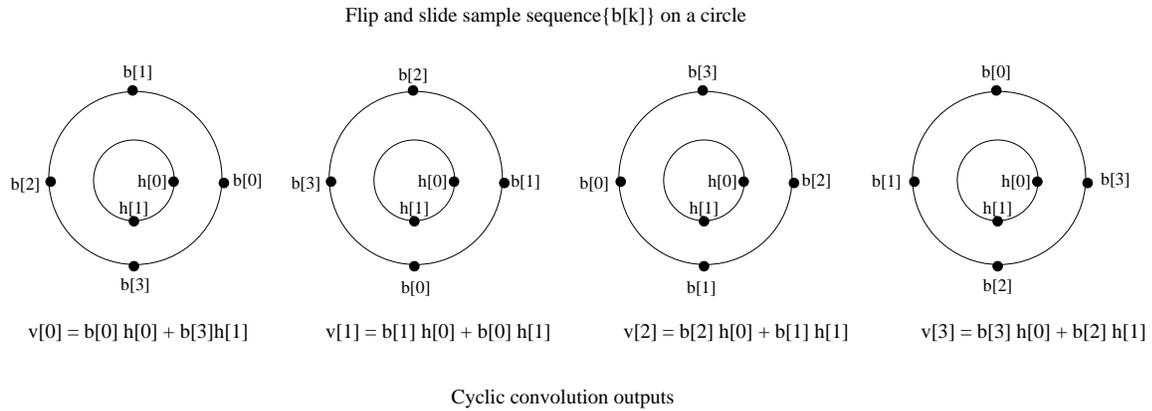
Figure 8.10: Example of cyclic convolution. Time progresses clockwise on the circle. The sequence  $\{b[k]\}$  is flipped, and hence goes counter-clockwise. We then “slide” this flipped sequence clockwise in order to compute successive outputs. Clearly, the output is periodic with period  $N = 4$ .
