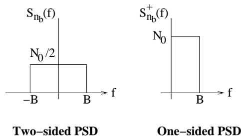
Figure 5.22: The PSD of baseband white noise.
