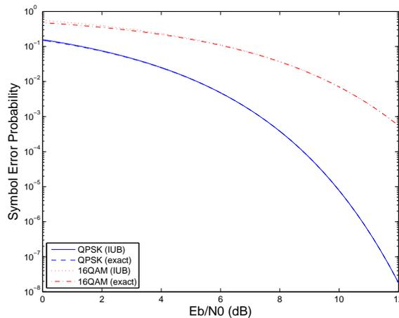
Figure 6.25: Symbol error probabilities for QPSK and 16QAM.
