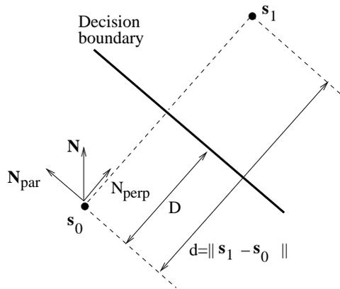
Figure 6.18: When making an ML decision between  $\mathbf{s}_0$  and  $\mathbf{s}_1$ , the decision boundary is at distance  $D = d/2$  from each signal point, where  $d = \|\mathbf{s}_1 - \mathbf{s}_0\|$  is the Euclidean distance between the two points.
