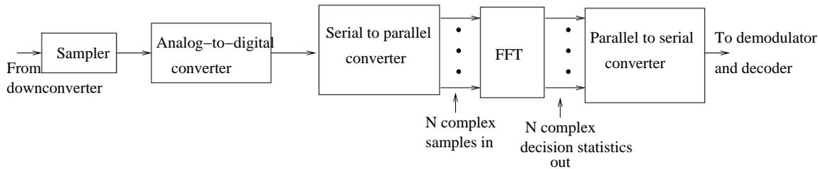
Figure 8.13: DSP-centric implementation of an OFDM receiver. Carrier and timing synchronization blocks are not shown.
