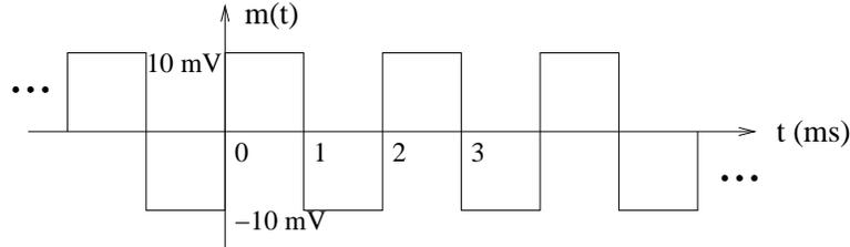
Figure 3.50: Message signal for Problems 3.21 and 3.22.
