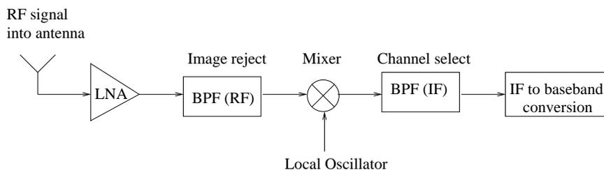
Figure 3.28: Generic block diagram for a superhet receiver.
