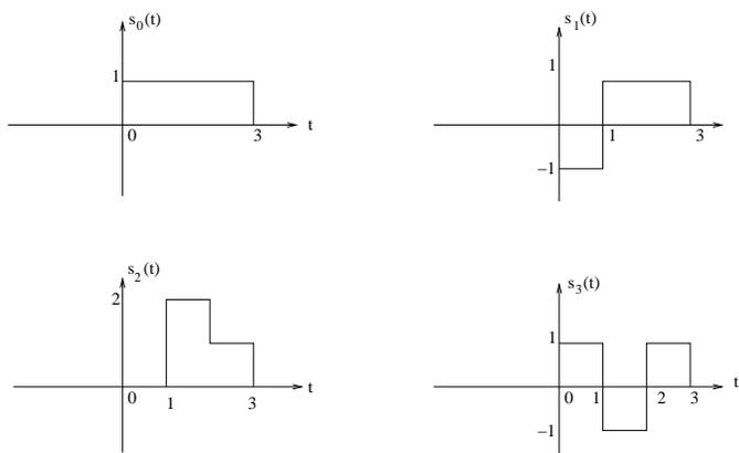
Figure 6.5: Four signals spanning a three-dimensional signal space
