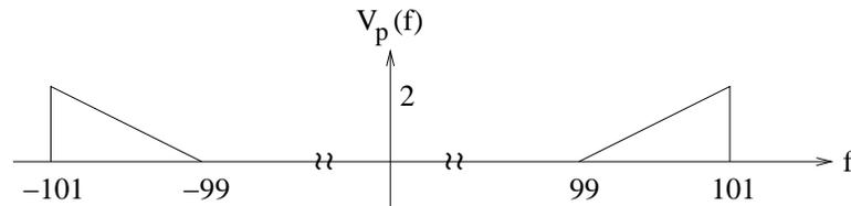
Figure 2.31: Sketch of passband spectrum for Example 2.8.4.
