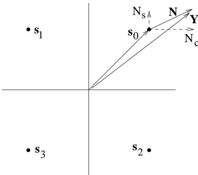
Figure 6.10: A signal space view of QPSK. In the scenario shown,  $\mathbf{s}_0$  is the transmitted vector, and  $\mathbf{Y} = \mathbf{s}_0 + \mathbf{N}$  is the received vector after noise is added. The noise components  $N_c, N_s$  are i.i.d.  $N(0, \sigma^2)$  random variables.
