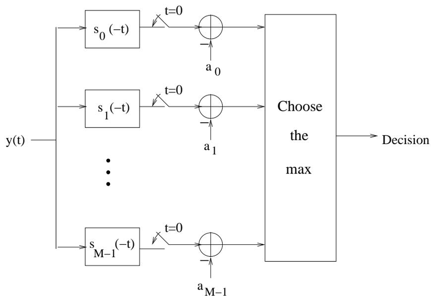
Figure 6.12: An alternative implementation for the optimal receiver using a bank of matched filters. For the ML rule, the constants  $a_i = \|s_i\|^2/2$ ; for the MPE rule,  $a_i = \|s_i\|^2/2 - \sigma^2 \log \pi_i$ .
