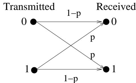
Figure 7.7: Binary symmetric channel with crossover  $p$ .
