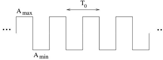
Figure 2.18: Square wave with period  $T_0$ .
