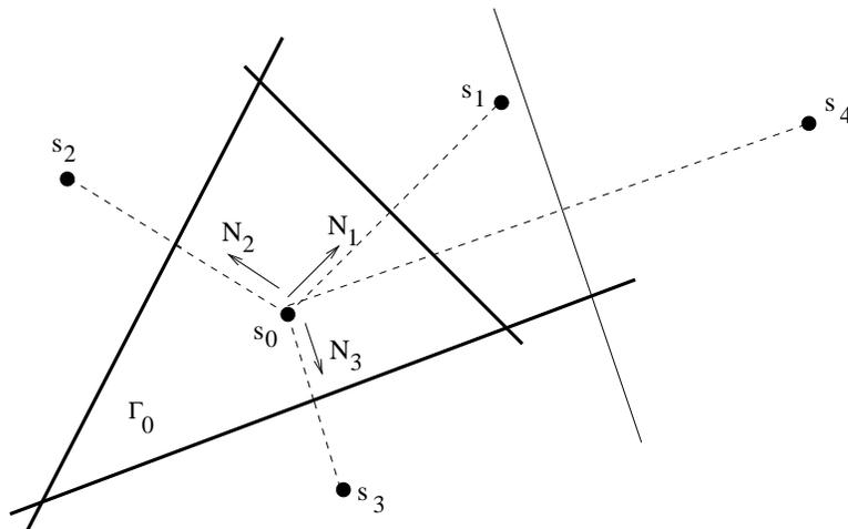
Figure 6.23: The noise random variables  $N_1, N_2, N_3$  which can drive the received vector outside the decision region  $\Gamma_0$  are correlated, which makes it difficult to find an exact expression for  $P_{e|0}$ .
