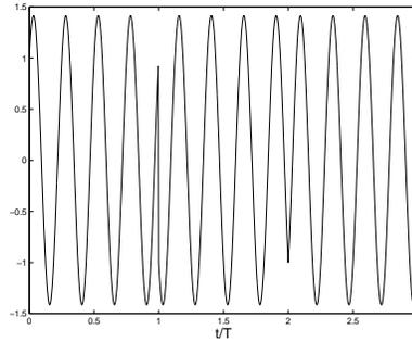
Figure 4.3: QPSK illustrated for  $f_c = \frac{4}{T}$ , with symbol sequences  $\{b_c[n]\} = \{+1, -1, -1\}$  and  $\{b_s[n]\} = \{-1, +1, -1\}$ . The phase of the passband signal is  $-\pi/4$  in the first symbol interval, switches to  $3\pi/4$  in the second, and to  $-3\pi/4$  in the third.
