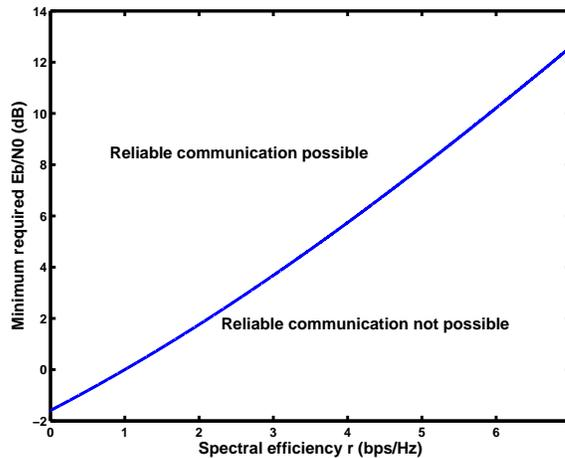
Figure 7.6: Power-bandwidth tradeoffs over the AWGN channel.
