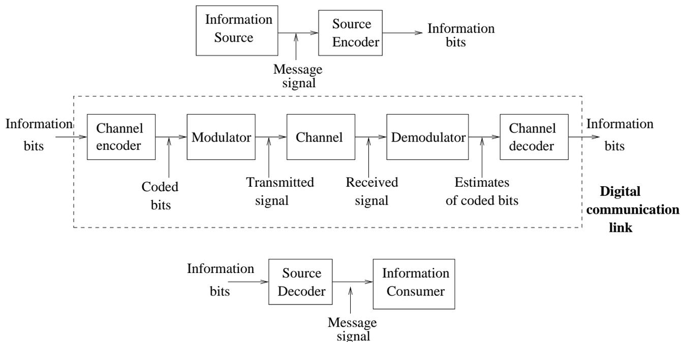
Figure 1.2: Components of a digital communication system.
