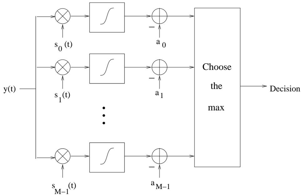
Figure 6.11: The optimal receiver for an AWGN channel can be implemented using a bank of correlators. For the ML rule, the constants  $a_i = \|s_i\|^2/2$ ; for the MPE rule,  $a_i = \|s_i\|^2/2 - \sigma^2 \log \pi_i$ .
