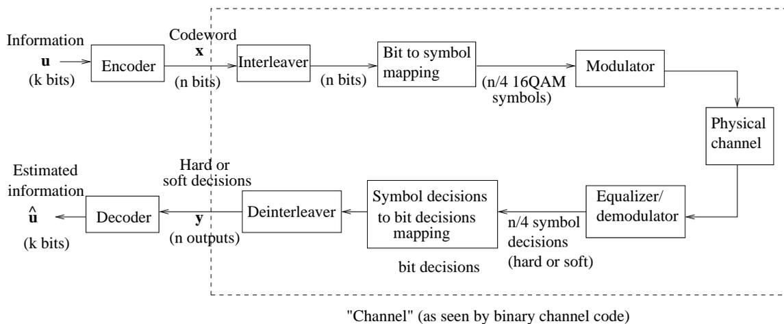
Figure 7.4: An example of bit interleaved coded modulation.
