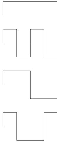
Figure 4.18: Walsh-Hadamard codes for 4-ary orthogonal modulation.
