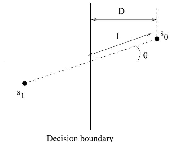
Figure 6.26: Performance analysis for BPSK with phase offset.
