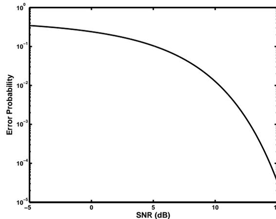
Figure 5.14: Probability of error versus SNR for on-off-keying.
