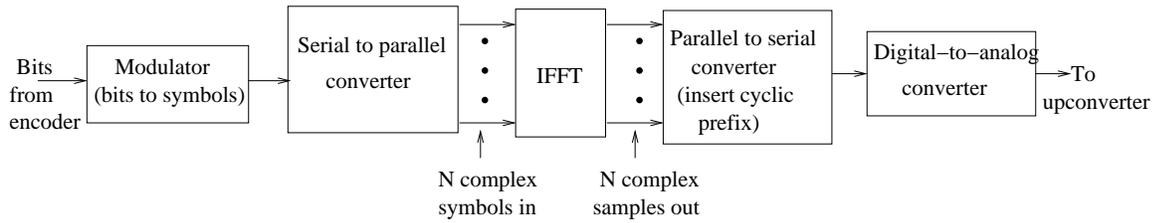
Figure 8.9: DSP-centric implementation of an OFDM transmitter.
