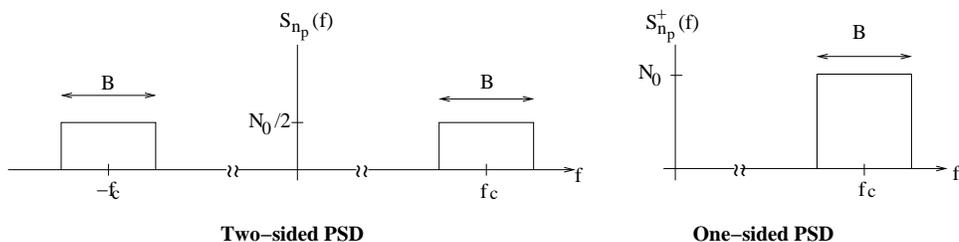
Figure 5.21: The PSD of passband white noise is flat over the band of interest.
