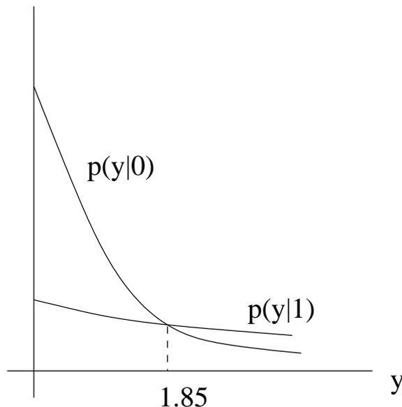
Figure 6.1: Hypothesis testing with exponentially distributed observations.
