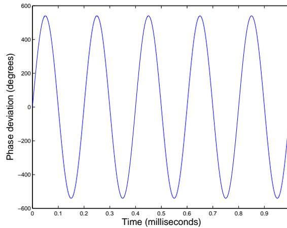
Figure 3.48: Phase deviation of FM signal for Problem 3.14.
