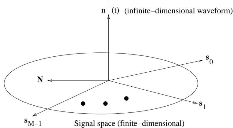
Figure 6.9: Illustration of signal space concepts. The noise projection  $n^\perp(t)$  orthogonal to the signal space is irrelevant. The relevant part of the received signal is the projection onto the signal space, which equals the vector  $\mathbf{Y} = \mathbf{s}_i + \mathbf{N}$  under hypothesis  $H_i$ .
