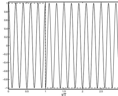
Figure 4.2: BPSK illustrated for  $f_c = \frac{4}{T}$  and symbol sequence  $+1, -1, -1$ . The solid line corresponds to the passband signal  $u_p(t)$ , and the dashed line to the baseband signal  $u(t)$ . Note that, due to the change in sign between the first and second symbols, there is a phase discontinuity of  $\pi$  at  $t = T$ .
