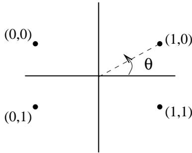
Figure 6.38: Signal constellation with unequal error protection (Problem 6.26).
