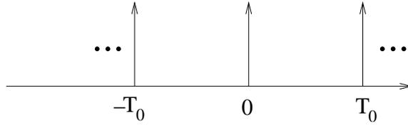
Figure 2.19: An impulse train of period  $T_0$ .
