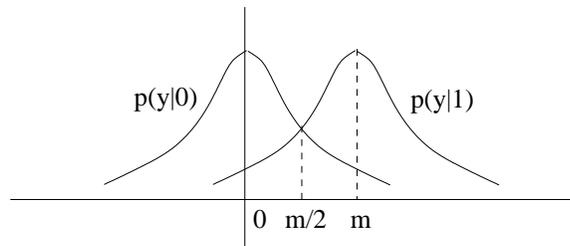
Figure 6.2: Conditional densities for the basic Gaussian example.
