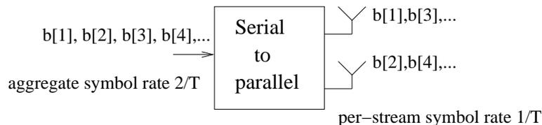
Figure 8.23: For spatial multiplexing, the transmitter may take a sequence of incoming symbols  $\{b[n]\}$ , and do a serial-to-parallel conversion to map them to subsequences to be transmitted from the different antennas. In the example shown, the odd symbols are transmitted from antenna 1, and the even symbols from antenna 2. The aggregate symbol rate is twice the per-stream symbol rate.
