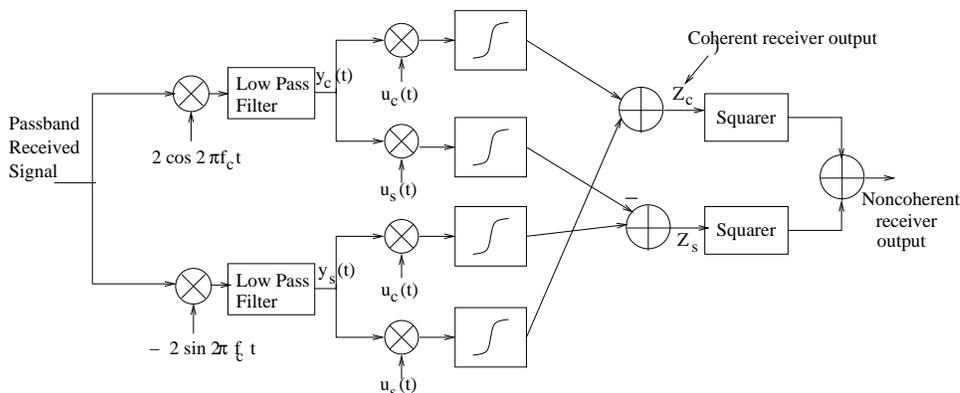
Figure 4.17: Structure of coherent and noncoherent receivers.
