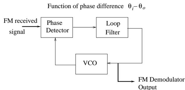
Figure 3.35: The PLL is an FM demodulator.
