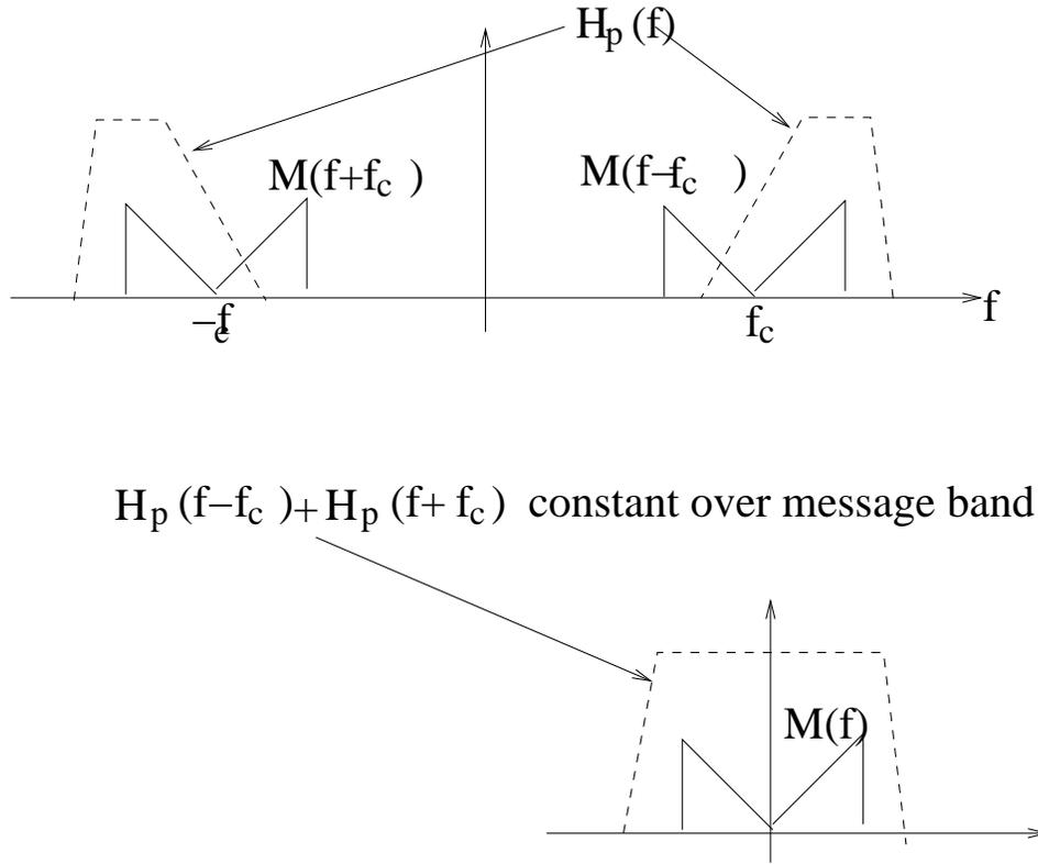
Figure 3.17: Relevant passband and baseband spectra for VSB.
