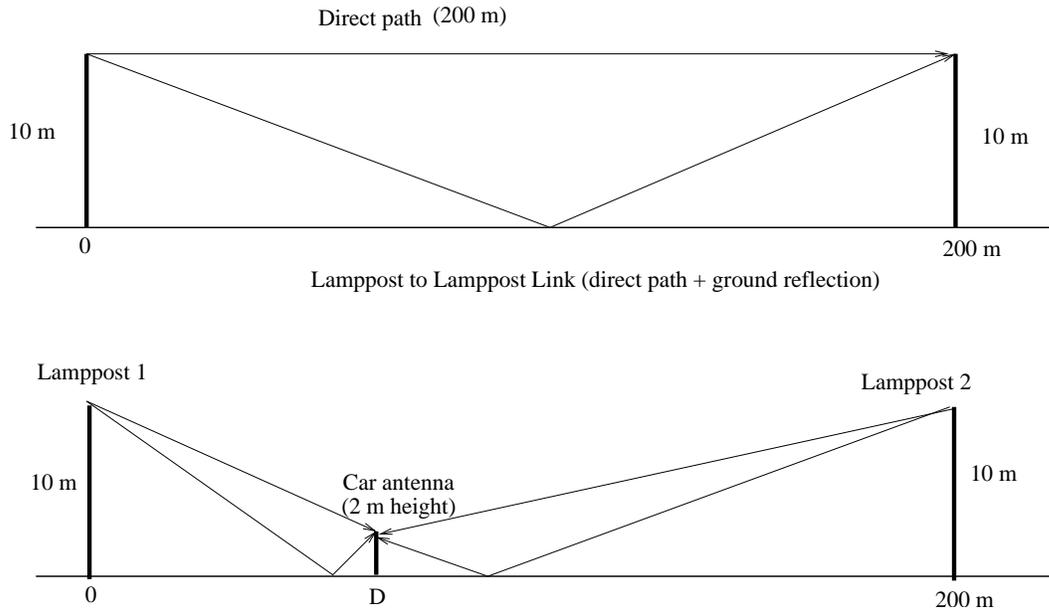
Figure 2.40: Links in a lamppost-based network.
