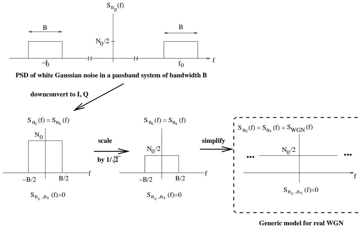
Figure 5.24: We scale the complex envelope for both signal and noise by  $\frac{1}{\sqrt{2}}$ , so that the I and Q components of passband WGN can be modeled as independent WGN processes with PSD  $N_0/2$ .
