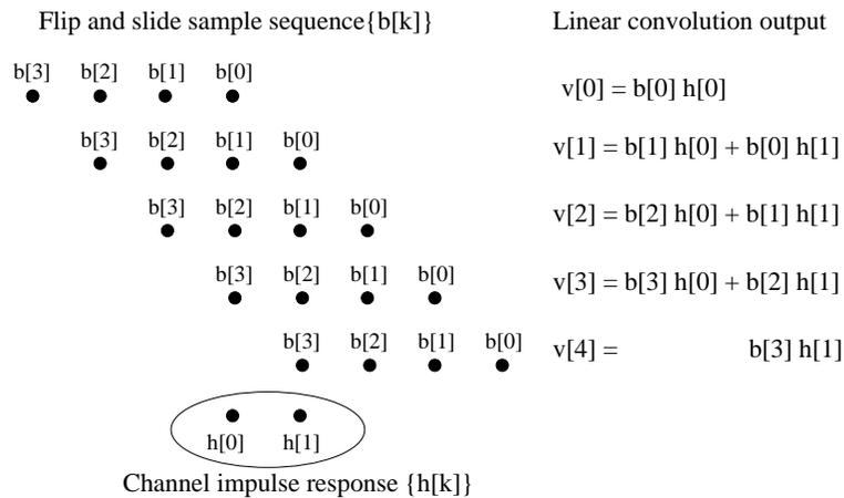
Figure 8.11: Linear convolution of the two sequences in Figure 8.10 leads to an aperiodic sequence of length  $2 + 4 - 1 = 5$ . Note that the outputs at times 1,2 and 3 coincide with the outputs of the corresponding cyclic convolution.
