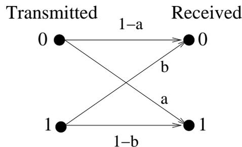
Figure 5.2: Conditional probabilities modeling a binary channel.
