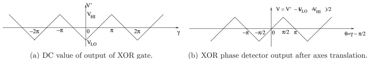
Figure 3.34: Response for the XOR phase detector.
