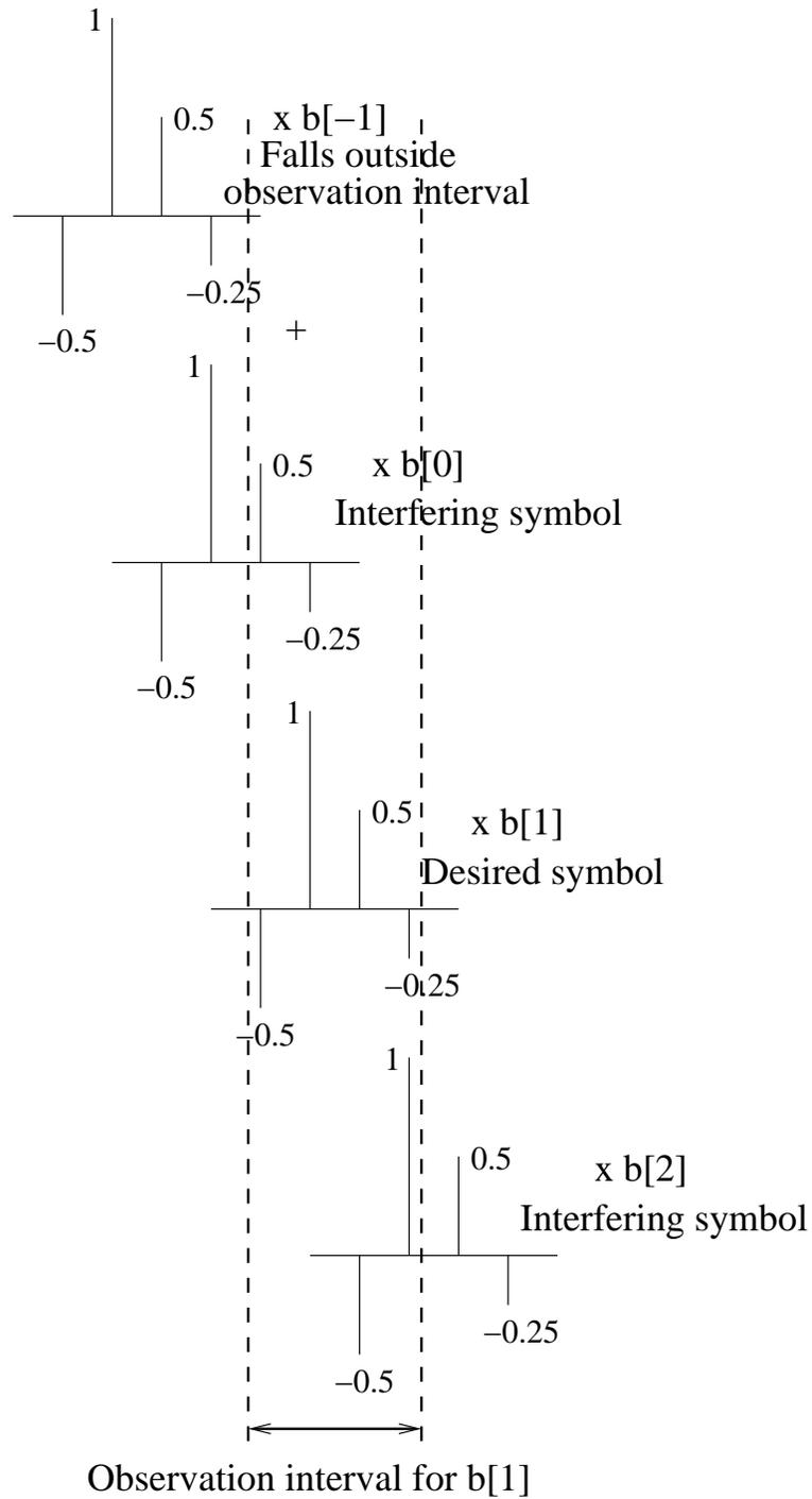
Figure 8.7: The observation interval used to make a decision on  $b[1]$  sees contributions from the desired symbol  $b[1]$  and interfering symbols  $b[0]$  and  $b[2]$ . Comparing with Figure 8.6, the roles of the symbols has shifted by one.
