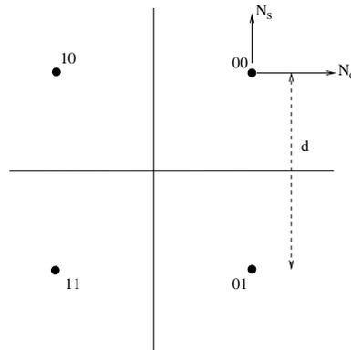
Figure 6.28: QPSK with Gray coding.
