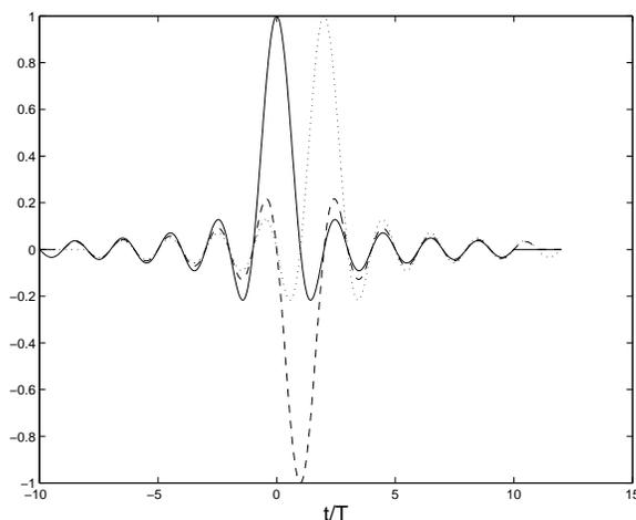
Figure 4.7: Three successive sinc pulses (each pulse is truncated to a length of 10 symbol intervals on each side) modulated by  $+1, -1, +1$ . The actual transmitted signal is the sum of these pulses (not shown). Note that, while the pulses overlap, the samples at  $t = 0, T, 2T$  are equal to the transmitted bits because only one pulse is nonzero at these times.
