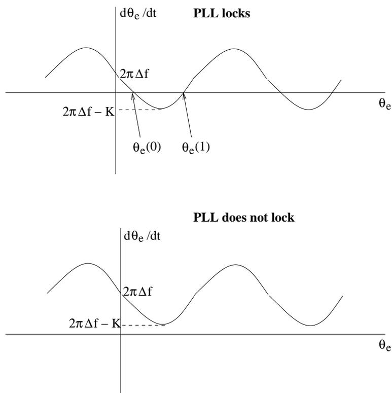
Figure 3.39: Phase plane plot for first order PLL.
