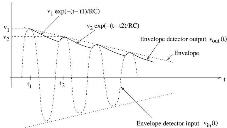
Figure 3.9: The relation between the envelope detector output  $v_{out}(t)$  (shown in bold) and input  $v_{in}(t)$  (shown as dashed line). The output closely follows the envelope (shown as dotted line).
