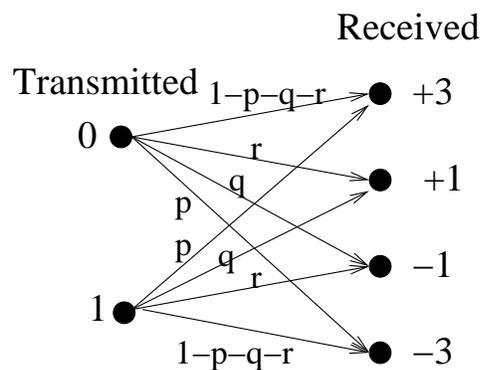
Figure 5.27: Two-input four-output channel for Problem 5.6.
