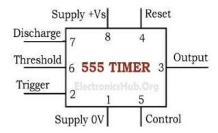
Pin Diagram of 555 Timer Image Source: ElectronicsClub.info/555timer.htm IC 555 timer is a renowned device in the field of electronics, although the majority of the people does not have any information regarding the internal circuitry as well as about the pins present on the IC. So here I have tried to explain the working of this IC so that you can build many projects around it and do your experiments.
