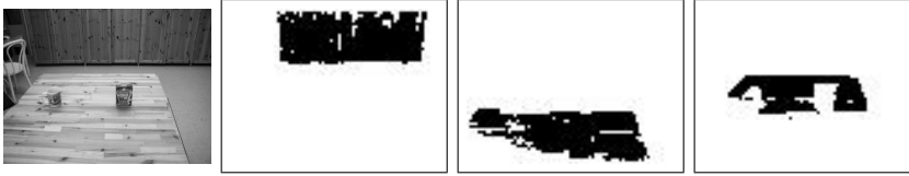
Figure 5.4: The left most image result in three mean-shift segments with r=0.15 , s=3
