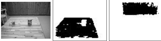
Figure 5.5: The left most image result in two mean-shift segments with r=0.22 , s=4
