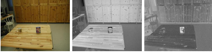
Figure 5.2: Raw image, U-, and V-feature map at the color node
