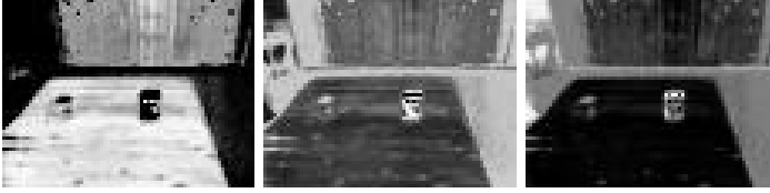
Figure 5.10: Gaussian Mixture Models, left to right image correspond to probability to fit first, second, and third Gaussian model
