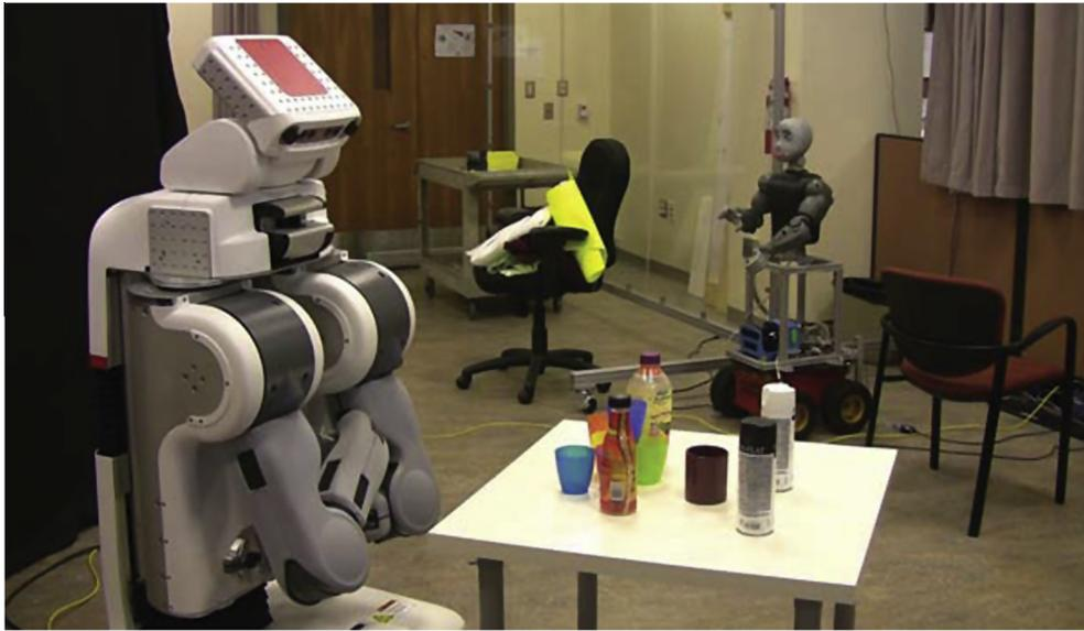
Fig. 8. PR2 robot acquiring data from a table top. The robot is able to position itself anywhere around the table.
