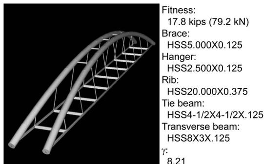
Fig. 7. A representative example of the stiff-rib solution type
