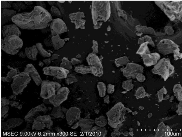
**Figure3:** Sem Image For 10% Tungsten Carbide With Aluminum
