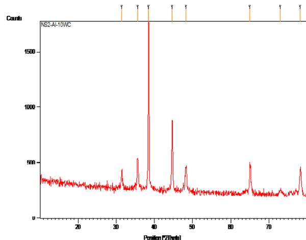
**Figure6:** XRD Test For 10% Wc With Al
