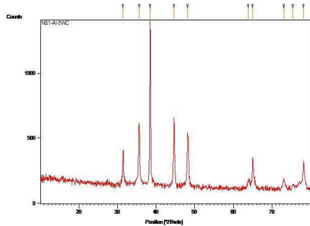
**Figure5:** XRD Test For 5% Wc With Al
