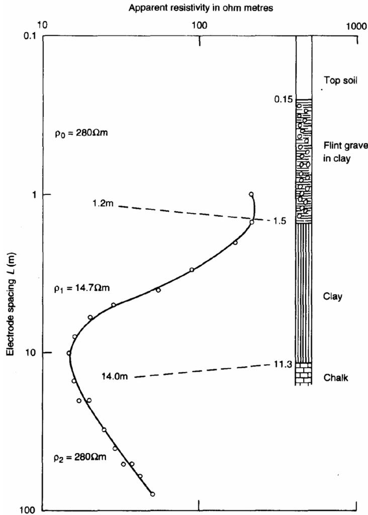
**Fig. 4.13** Interpretation of electrical resistivity sounding data.
