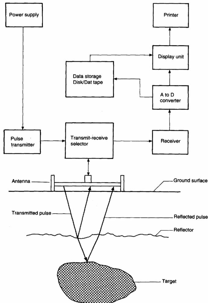
**Fig. 4.18** Schematic diagram showing the operation of a ground penetrating radar (GPR) system.
