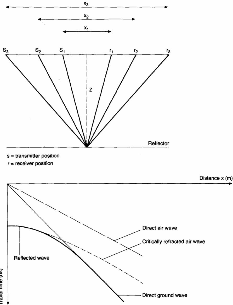
**Fig. 4.22** Illustration of CMP sounding.
