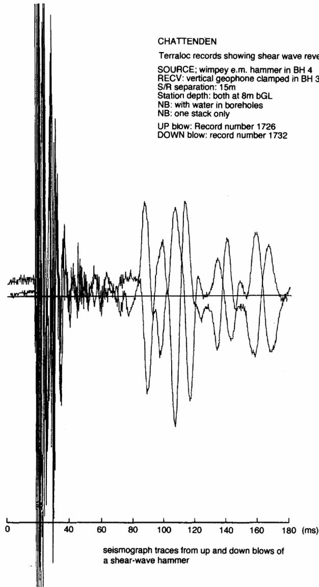
**Fig. 4.36** Shear wave reversals on two traces recorded by a signal-enhancement seismograph.
