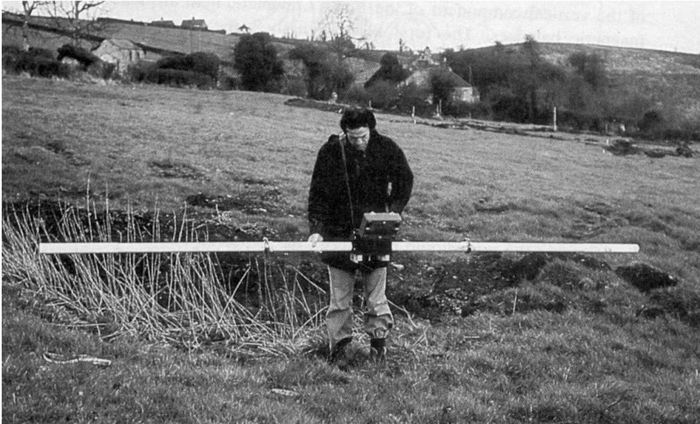
**Fig. 4.3** Geonics EM31 ground conductivity meter
