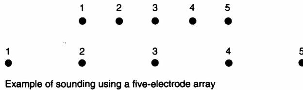
Fig. 4.10 Principles of sounding with Offset Wenner five-electrode array.
