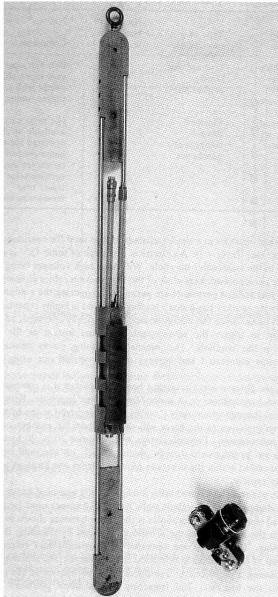
**Fig. 4.32** Bison shear wave hammer.
