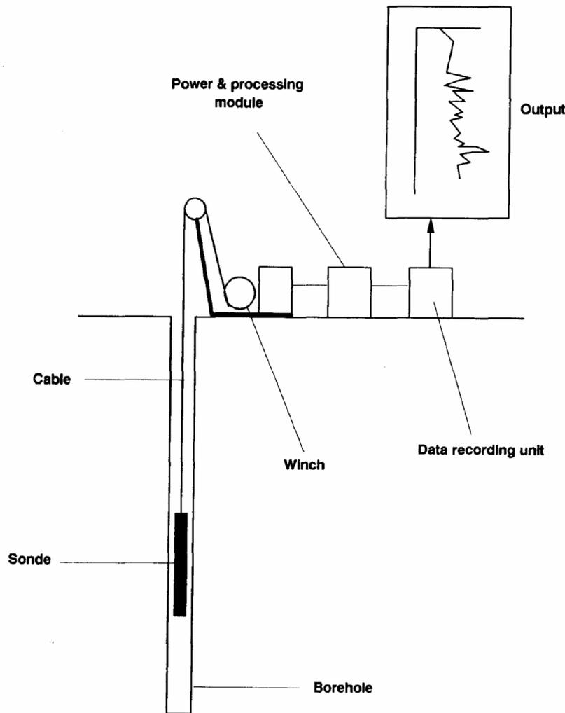
**Fig. 4.16** Elements of a geophysical borehole logging system.
