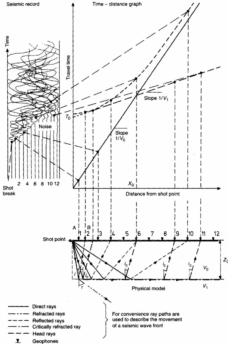
**Fig. 4.34** Seismic refraction using P-wave events (first arrivals).
