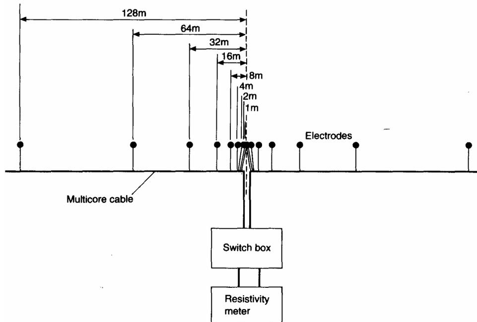
**Fig. 4.11** Arrangement for Wenner Offset sounding using multicore cable and switch box for  $a=0.5, 1, 2, 4, 8, 16, 32$  and  $64$ m.
