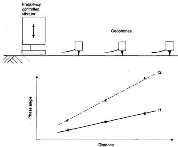
**Fig. 4.41** The surface wave technique.
