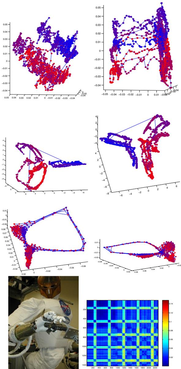
Figure 4. 3D embeddings of 57D Robonaut sensor data from PCA (top row), Isomap using 20 K-NN (top middle row), and continuous ST-Isomap using 3 KNTN (bottom middle row). An image of the NASA Robonaut and the distance matrix from continuous ST-Isomap (bottom). In each plot, sequentially adjacent points are connected by a blue line and temporal order is color coded from blue to red.
