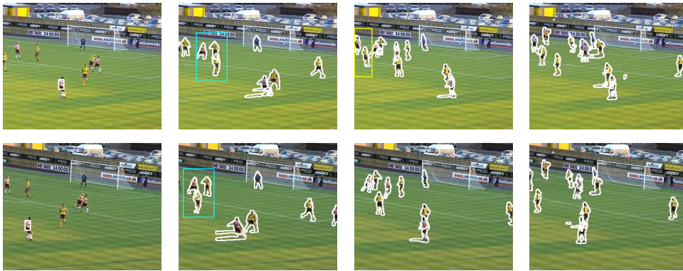
Figure 5: Two view example: the top row shows extracts from one sequence, while the bottom row the same time-instants from a different viewpoint. Note: (i) automatic creation of new layers from a single layer (leftmost) to multiple layers; (ii) new layers being created as players enter one field of view (eg, yellow box, third column); (iii) correct treatment of occlusion (eg, cyan box, second column).
