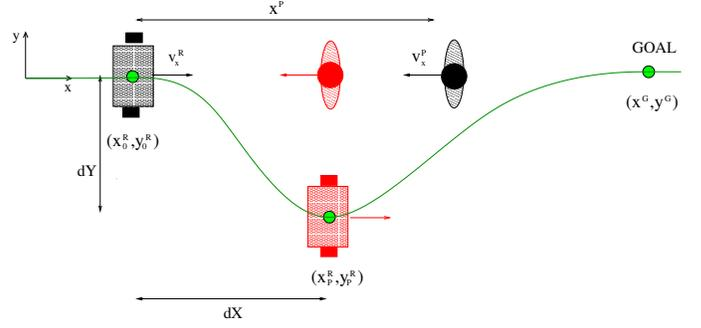
Fig. 5. Desired trajectory for the passage maneuver. The distance of the robot from the person is maximum when it is passing her/him (red).
