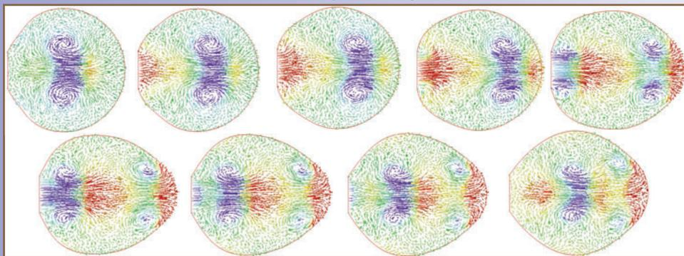
**Figure 1:** Inflation of a balloon: velocity vectors colored by air pressure, from 2 to 4 sec. This figure appears as Fig. 7.12, p. 180, in the book
