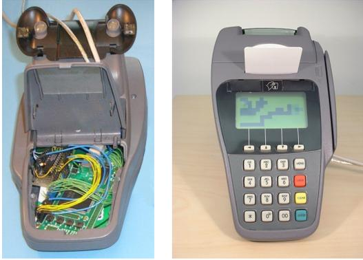
Figure 6. Modified Chip and PIN terminal, playing Tetris
