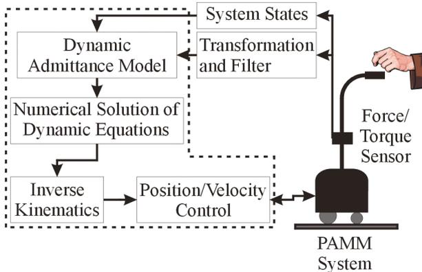
Figure 3. User Control System Diagram
