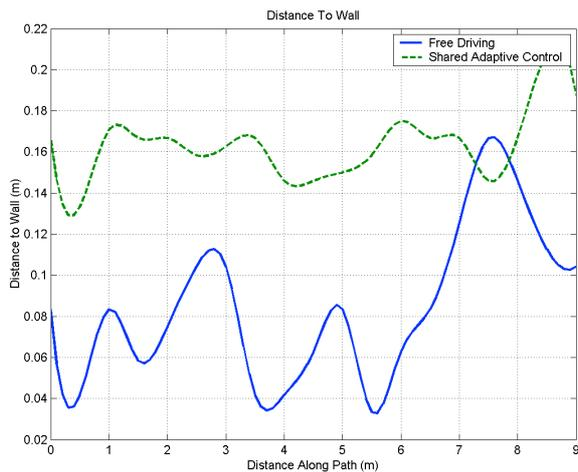
Figure 7. Distance to Wall for Free Driving and Shared Adaptive Control for a Single Subject.
