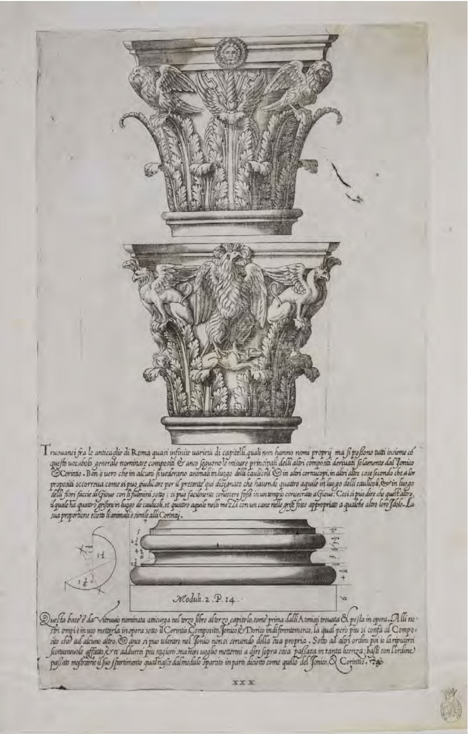
Cat. 20.5 Giacomo Barozzi da Vignola Italian, 1507–1573 Regola delli cinque ordini d’architettura , Rome: 1563, Plate XXX Composite order, two ancient capitals and a base Engraving, 13¾ x 8⅞ in, 34.92 x 20.57 cm Courtesy of Avery Architectural and Fine Arts Library, Columbia University, Speculum Romanae Magnificentiae Collection, 1951.001.00404
