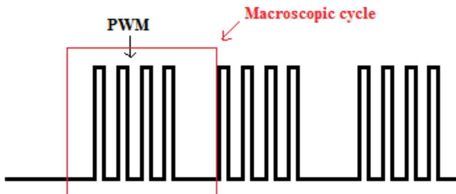
Figure 5, software level calibration of motor speed. PWM signal is sent to the motors during part of the time in the macroscopic cycle. The motors are actually repeating start and stop in each macroscopic cycle. This will cause the robot to move slower.
