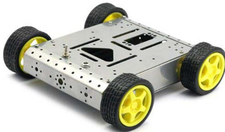
Figure 4, aluminum four wheel drive arduino platform
