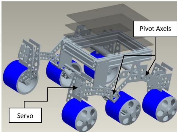
Figure-1: MIL Rover ProE model
