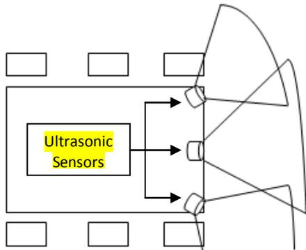
Figure-5: Ultrasonic sensors for obstacle avoidance (exaggerated beam)
