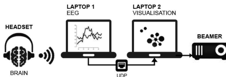
Figure 16. Hardware setup. Laptop 1 analyzes the EEG readings from the wireless headset and sends the SMA values to laptop 2, which renders the visualization using NODEBOX FOR OPENGL.
