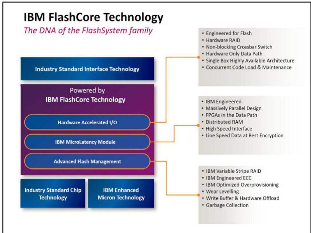
Figure 3 IBM FlashCore technology
