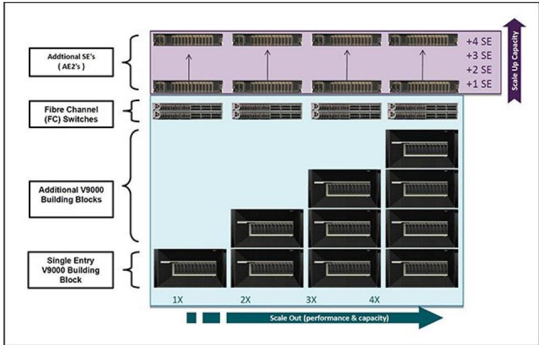
Figure 6 FlashSystem V9000 scalable capacity
