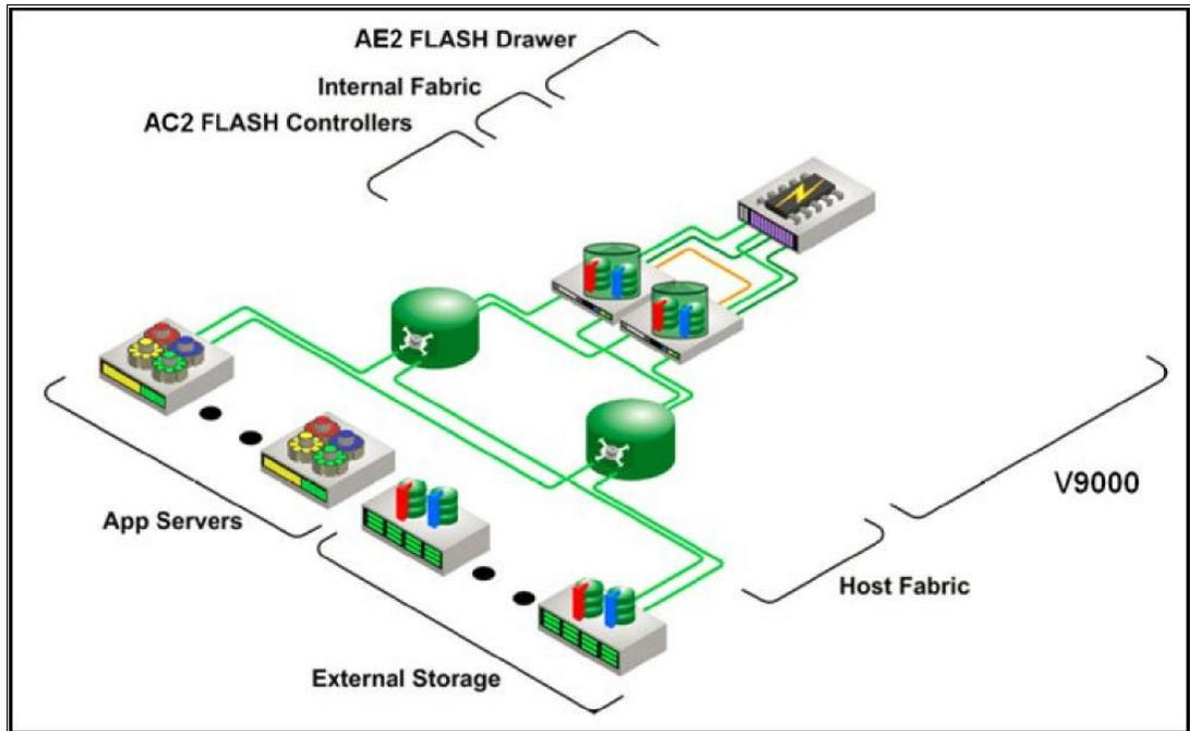
Figure 7 FlashSystem V9000: Generalized view of host connectivity topology
