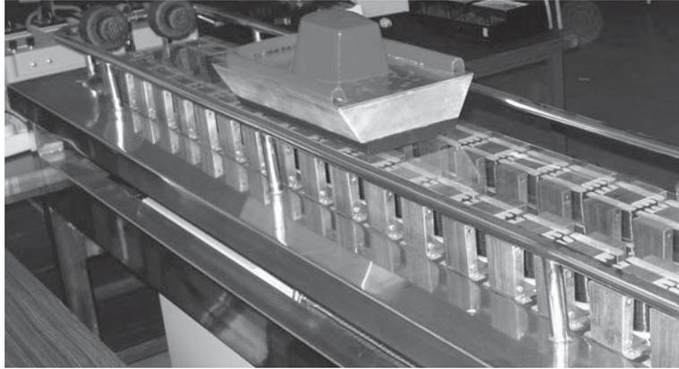
**FIGURE 34.26** Flat LIM with transverse magnetic flux, salient poles, and nonferromagnetic secondary propelled, suspended, and stabilized electro-dynamically. (From Gieras, J.F. et al., Analytical calculation of electro-dynamic levitation forces in a special-purpose linear induction motor, *International Electric Machines and Drives Conference (IEMDC'11)*, Niagara Falls, Ontario, Canada, 2011 [on CD-ROM].)
