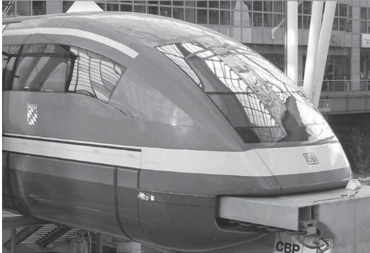
**FIGURE 34.19** Transrapid 09 maglev train driven by LSMs with electromagnetic excitation. (Photo courtesy of Thyssen Transrapid System GmbH, Munich, Germany.)
