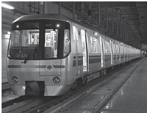
**FIGURE 34.30** Toei Oedo subway line in Tokyo driven by single-sided LIMs.
