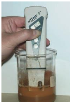
Figure 4. Measuring the pH of the supernatant with a pH meter.
