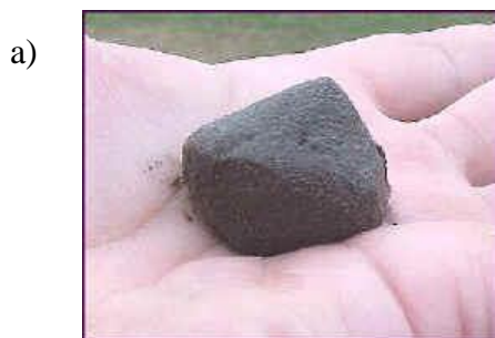
Figure 2. a) Picture showing initial addition of water to the soil and formation of a ball. b) Picture showing the formation of a soil ribbon.
