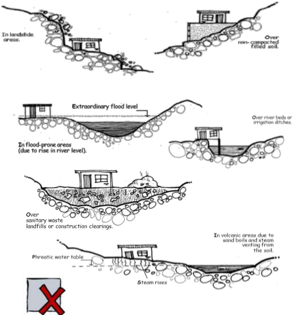
**Where not to build.** Examples of places where it is dangerous to build and where houses may easily be destroyed.
