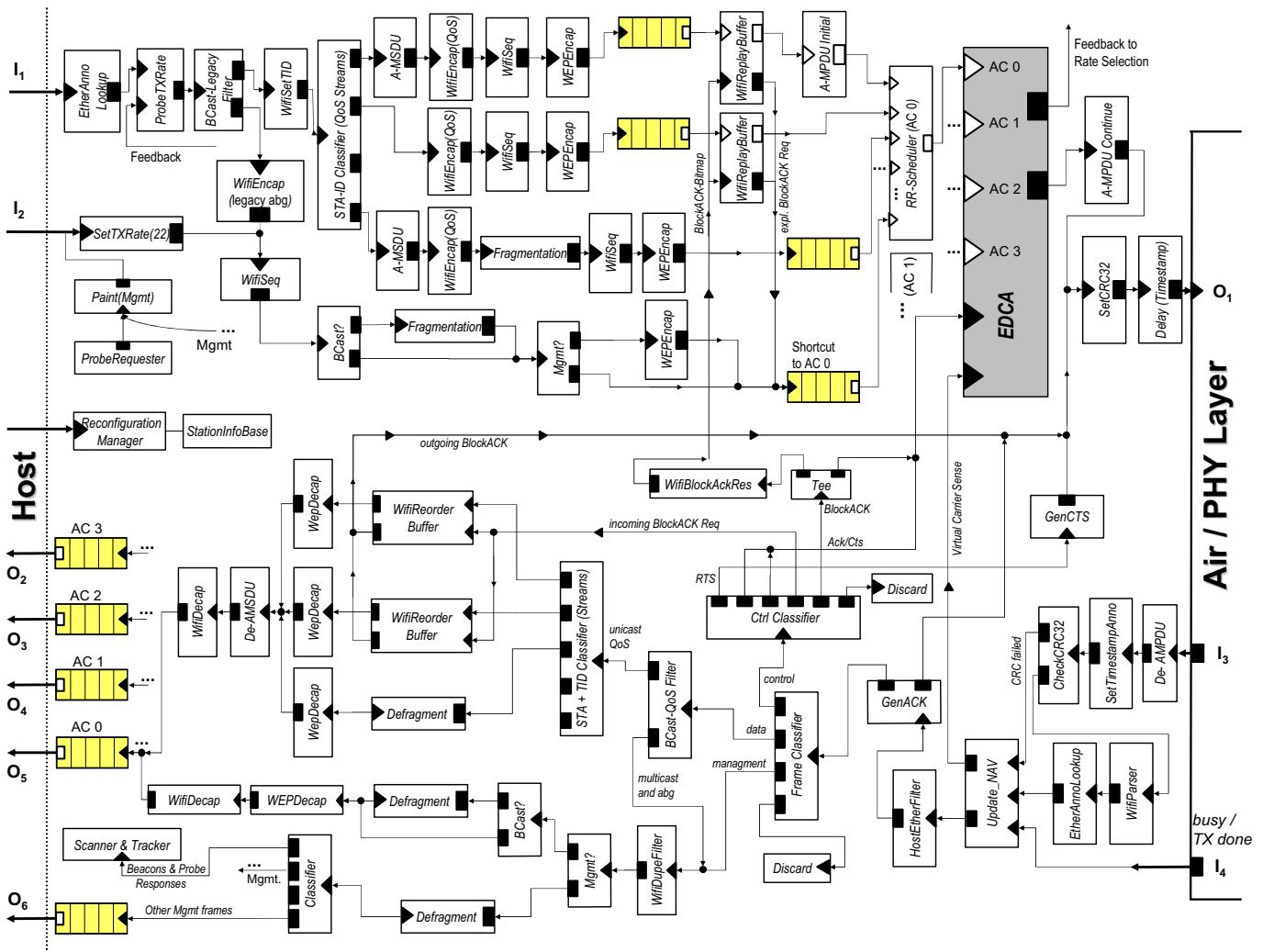
Fig. 1. Click model of a WLAN 802.11abg/en MAC with transmit paths in the upper half and receive paths below.
