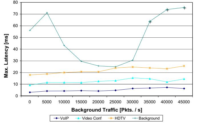
Fig. 2. Maximum end-to-end latencies in the QoS scenario as background traffic load is increased. The channel model's drop rate is 5%.
