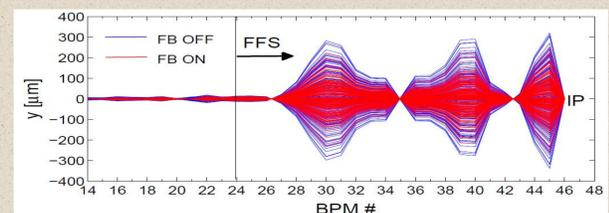
Vertical offset distribution at the IP for bunch 2 and 3 for 1000 pulses:
