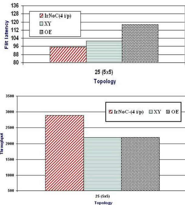
Fig 6: Performance comparison of irregular and regular (2D Mesh) NoC on the NoC simulation framework
