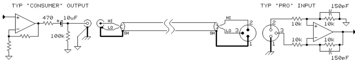
**CORRECT** Connection is Much Better - **Noise Rejection = 20 dB to 30 dB**
