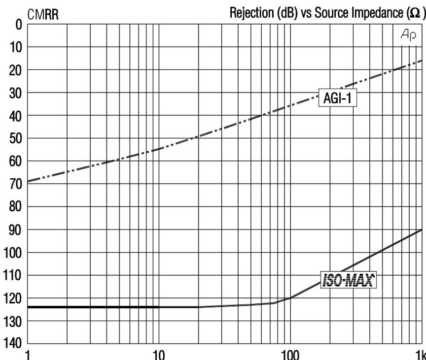
The plots at left compare the 60 Hz hum rejection performance of another typical active interface device, the now discontinued Sonance AGI-1 “audio ground isolator,” to that of an input-transformer based isolator. Over the consumer output impedance range of 200 Ω to 1 kΩ, the *active* isolator achieves only 15 to 30 dB of rejection while the ISO-MAX® CI-2RR isolator improves that by some 80 dB!
