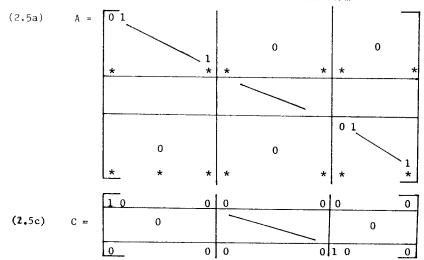
The p diagonal blocks of A and C are  $l_i \times l_i$  and  $1 \times l_i$  respectively.
