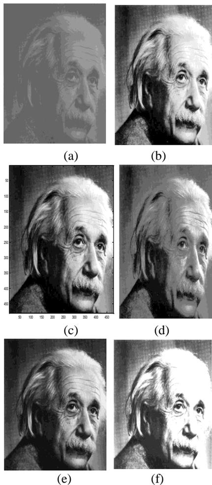
Figure 4. a) Original image b) SHE image c) BHE image d) RMSHE image using 8 sub block e) NOSHE image using 4 sub-block f) NOSHE image using 8 sub-blocks
