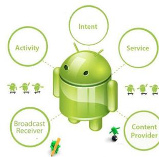
Figure 3. Android Application components
