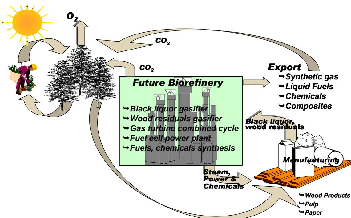
Figure S1. Future “biorefinery” concept based at a pulp and paper manufacturing facility.
