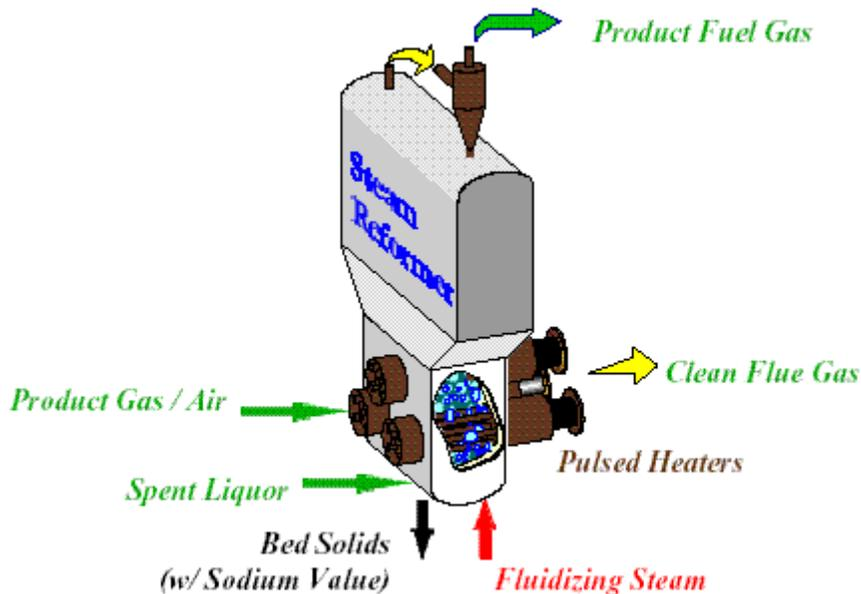
Figure 8. TRI black liquor gasification concept.
