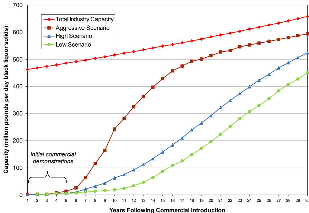
**Figure 24. Market penetration estimates used to assess energy and environmental impacts of BLGCC implementation in the United States.**
