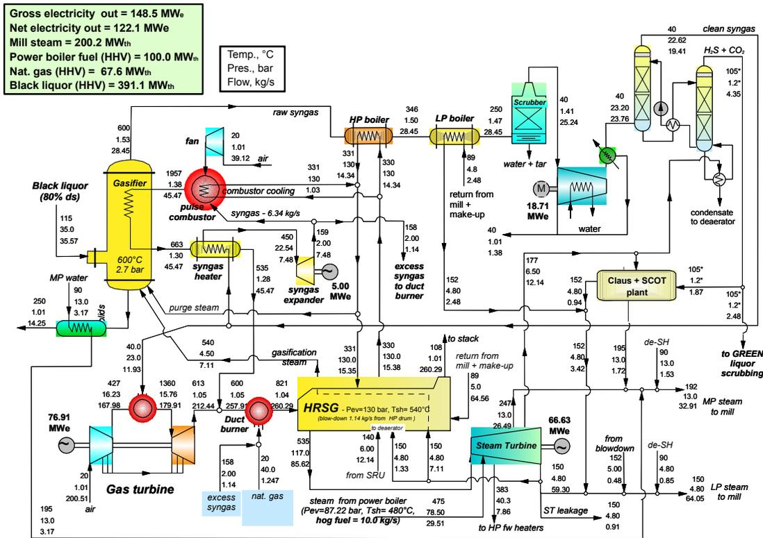
Figure S6. Energy/mass balance for BLGCC with low-temperature gasifier and mill-scale gas turbine.
