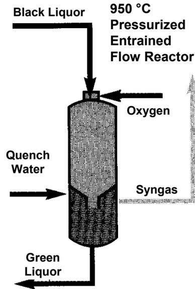
Figure 7. Chemrec black liquor gasification concept.
