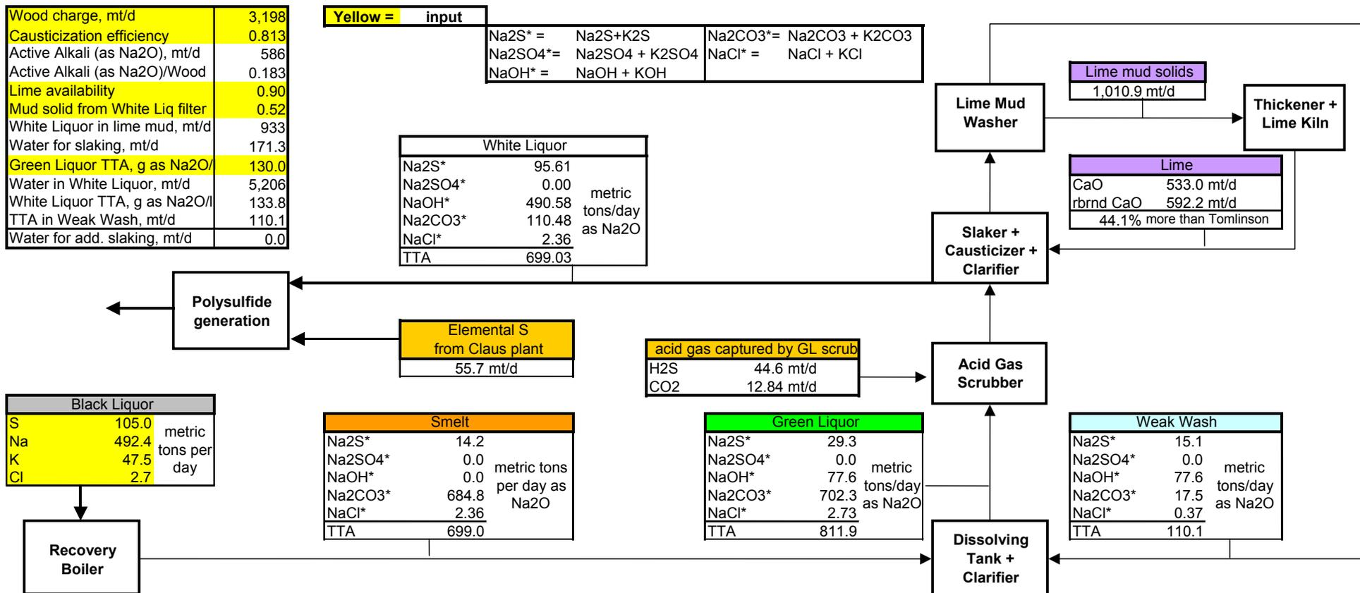
Figure A4. Estimate of causticization load for the low-temperature gasification case. TTA = Total Titratable Alkali.
