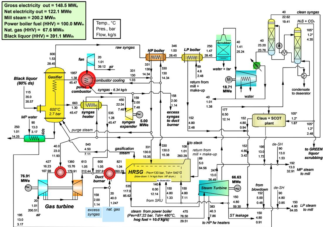
**Figure 12. Energy/mass balance for BLGCC with low-temperature gasifier and mill-scale gas turbine.**
