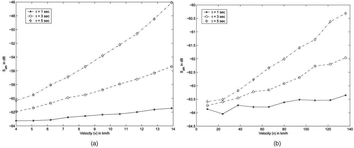
Fig. 10. RSS threshold ( $S_{ath}$ ) for different speed values when the OBS belongs to a: (a) microcellular system and (b) macrocellular system.
