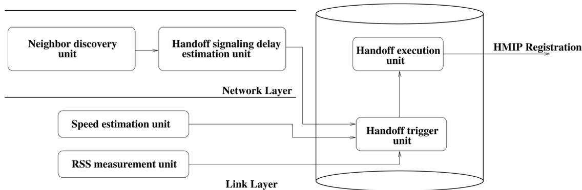
Fig. 6. The modules of cross-layer handoff management architecture.
