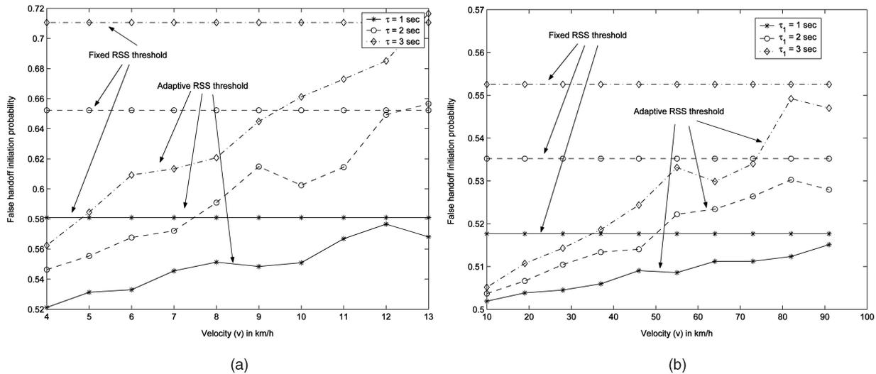
Fig. 14. Relationship between false handoff initiation probability of CHMP and speed when the OBS belongs to a: (a) microcellular system and (b) macrocellular system.
