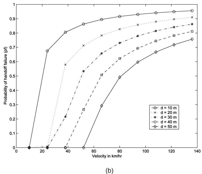
Fig. 4. Relationship between handoff failure probability and MT's speed: (a) for intrasystem handoff with  $\tau = 1$  sec and (b) for intersystem handoff with  $\tau = 3$  sec.
