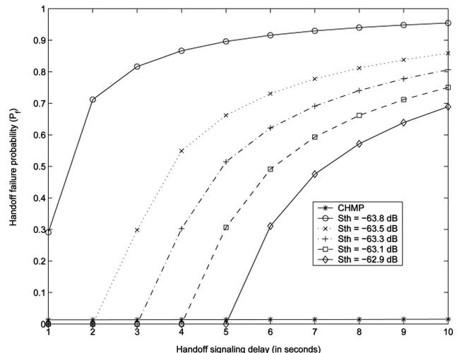
Fig. 13. Relationship between handoff failure probability of CHMP and handoff signaling delay.
