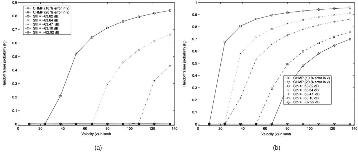
Fig. 12. Relationship between handoff failure probability of CHMP and speed when the OBS belongs to a macrocellular system: (a) intrasystem handoff scenario and (b) intersystem handoff scenario.
