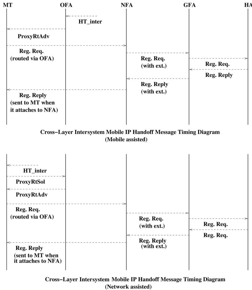
Fig. 9. Timing diagram for cross-layer intersystem HMIP handoff.
