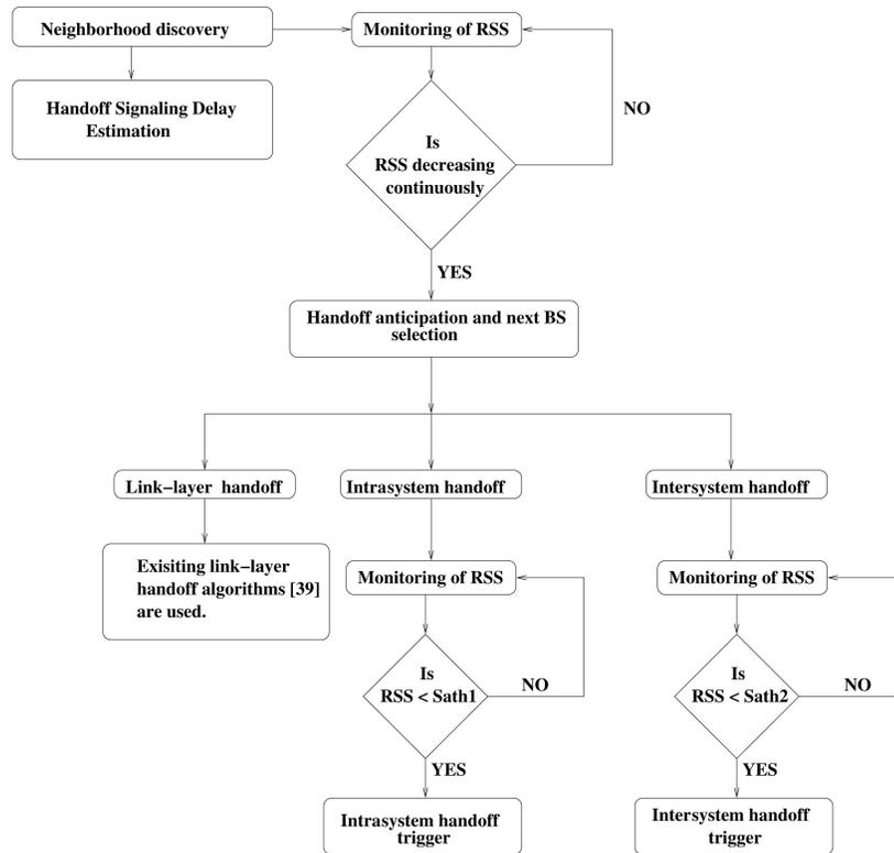
Fig. 7. Flow diagram of CHMP operation.
