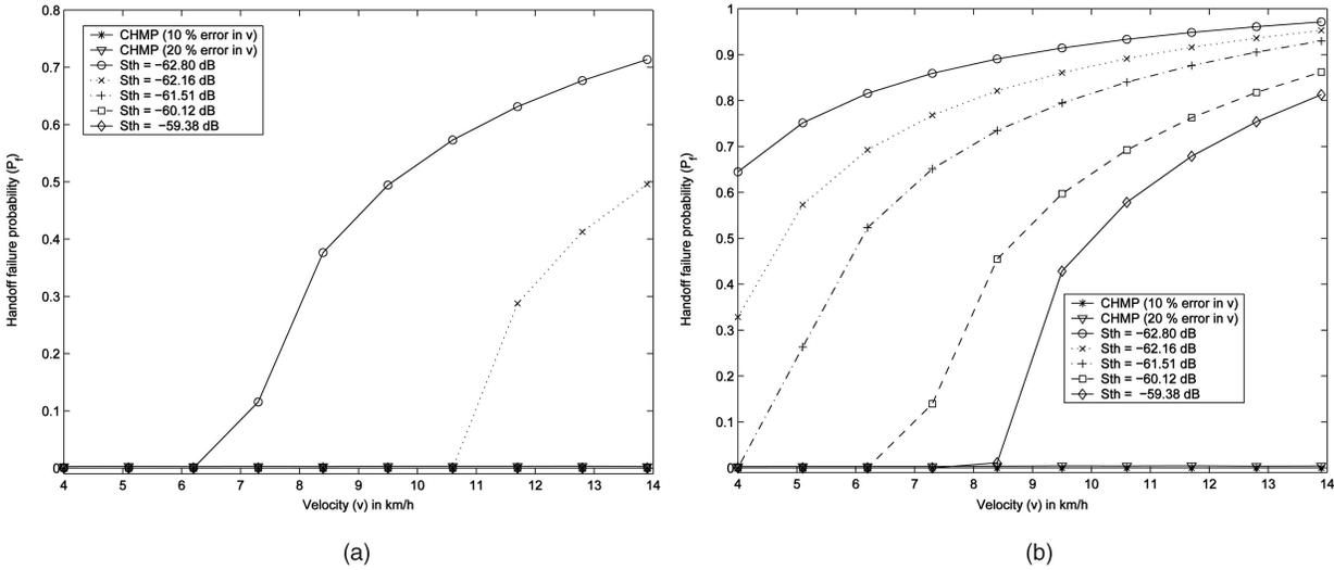
Fig. 11. Relationship between handoff failure probability of CHMP and speed when the OBS belongs to a microcellular system: (a) intrasystem handoff scenario and (b) intersystem handoff scenario.
