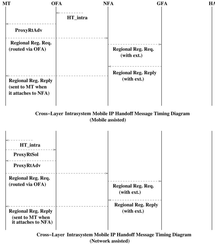
Fig. 8. Timing diagram for cross-layer intrasystem HMIP handoff.
