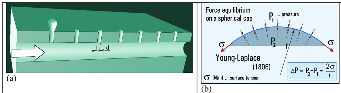
Figure 1 Instability of parallel percolation. (a) If one of the bubbles increases beyond the hemispherical shape, its growth becomes easier: air entering overcomes a lower pressure difference  $\Delta P$ . It grows at the expense of the other bubbles. (b) The basic reason: Young-Laplace surface tension law. Pressure difference across the air/water surface is inversely proportional to the curvature radius  $r$ .
