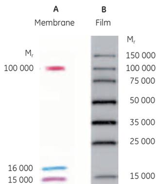
**Fig 3.6.** Amersham ECL DualVue Western Blotting Markers after electrophoresis on a 4-20% SDS-PAGE gel and transfer onto an Amersham Hybond™ ECL nitrocellulose membrane. Prestained indicator proteins are shown as a photograph of the membrane (A), together with tagged recombinant proteins after detection with Amersham ECL as a photograph of the film, following 1 min exposure (B).
