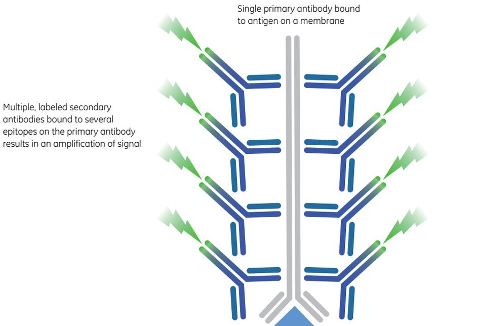
**Fig 5.1.** As multiple secondary antibodies conjugated to an enzyme or a fluorophore can bind to a single, specific primary antibody, the signal can be greatly amplified, contributing to the sensitivity of Western blotting.
