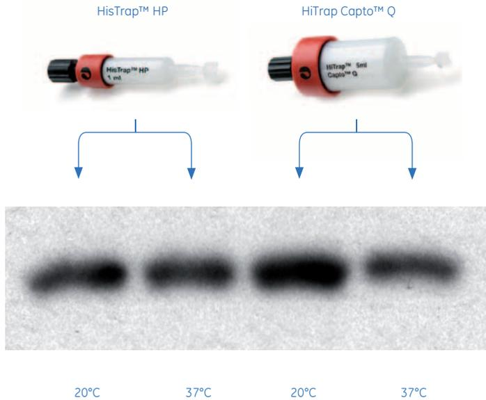
**Fig 9.1.** Detection of recombinant histidine-tagged GFP with Amersham ECL and Amersham Hyperfilm ECL, for comparison of protein yields after different induction temperatures (20°C or 37°C) and purification media (HisTrap HP (1 ml) or HiTrap Capto Q (5 ml) on ÄKTAexplorer™). A visual analysis of the results from this purification shows that the highest yield of histidine-tagged GFP was achieved using an induction temperature of 20°C and purification on HiTrap Capto Q.
