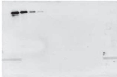
**Fig 4.3.** Comparison of blots following wet and semidry transfer. A two-fold dilution series of transferrin starting at 5  $\mu\text{g}$  was transferred to Hybond-P membranes (PVDF). Semidry transfer is less efficient for this particular protein than wet transfer; less protein throughout the dilution series is transferred, leading to reduced sensitivity.
