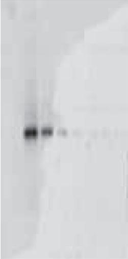
We recommend that you scan properly dried membranes (not partially dried or wet). Scanning dried membranes usually results in a more even background and a higher signal-to-noise ratio. The membrane shown here was not fully dried and the bands to the right are very weak.
