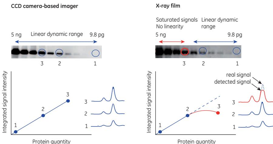
**Fig 8.2.** The advantage of using a CCD camera-based imager compared to X-ray film for signal detection. For the CCD camera-based system, all bands fall within the linear dynamic range of the system, whereas for film, the most intense bands (indicating more protein) are saturated, rendering quantitation impossible at this portion of the curve as the volume under the curve can no longer be determined.
