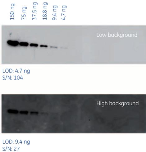
**Fig 8.8.** A two-fold serial dilution of actin detected on blots using Amersham ECL: Some important consequences of elevated background levels on signal quantitation. The signals shown in the upper panel were obtained using optimized antibody concentrations. No optimization was performed for the signals shown in the lower panel. The consequence is a higher background, which affects LOD and the signal-to-noise ratio.
