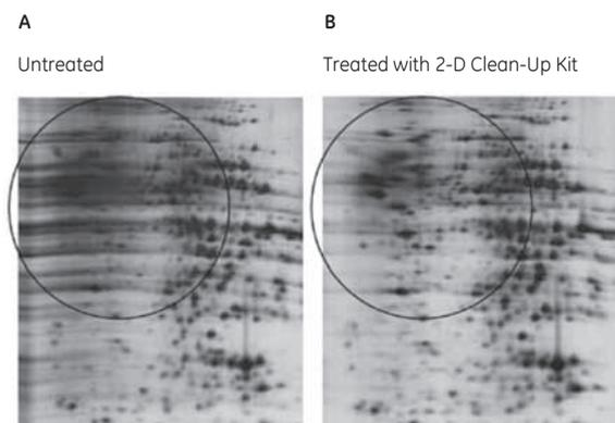
**Fig 2.2.** 2-D Clean-Up Kit eliminates most of the horizontal streaking caused by residual SDS.
