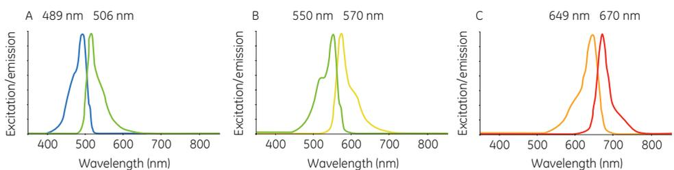
**Fig 6.8.** Excitation and emission spectra for fluorescent Amersham CyDyes (A) Cy2, (B) Cy3, and (C) Cy5. In each example, the effect of the light wavelength generating the maximum efficiency of excitation is shown.
