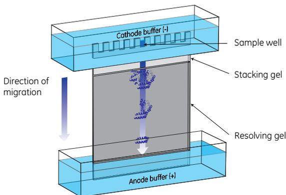
**Fig 3.1.** A vertical electrophoresis apparatus is set up with cathode (-) buffer in an upper chamber and anode (+) buffer in a lower chamber. Molecules in sample wells migrate toward the anode (+) in an electric field. After a set amount of time, the molecules will have migrated to positions based on their size, shape and charge. As an alternative to vertical electrophoresis systems, horizontal systems are also available.
