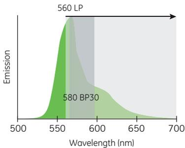
**Fig 7.3.** Emission filtering of Cy3 fluorescence using either a 580 BP30 filter (dark grey area) or a 560 LP filter (light and dark grey areas). BP = band pass. LP = long pass.
