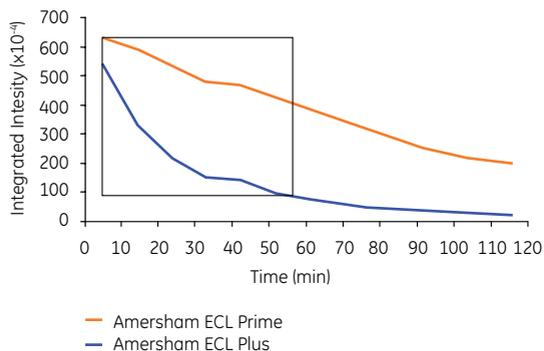
**Fig 6.7.** Signal stability over time. The signal duration of Amersham ECL Prime compared to an alternative chemiluminescent detection reagent. The high stability of Amersham ECL Prime provides a broader window of time in which higher sensitivity is maintained.
