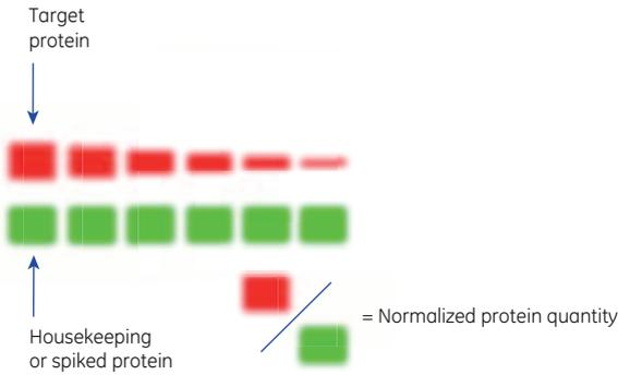
**Fig 8.4.** Illustration of how to normalize a target protein to a housekeeping or spiked protein. Initially, the intensity of each band is calculated using analysis software. The measured value for each target protein is then related to the corresponding value of the housekeeping or spiked protein.
