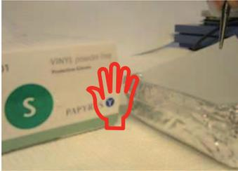
Use powder-free gloves when working with fluorescence detection.
