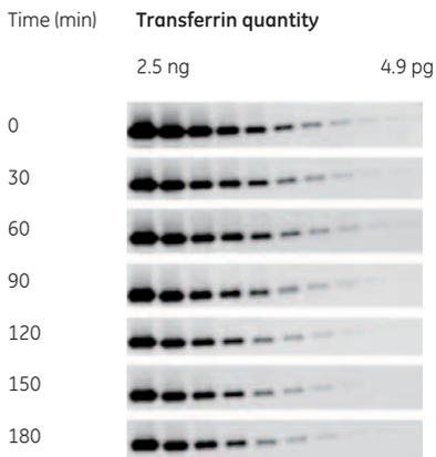
**Fig 6.6.** A two-fold dilution series of transferrin from 2.5 ng showing signal intensities at time points up to 3 h after the addition of Amersham ECL Prime reagent. Time 0 corresponds to 5 min post-reagent addition. The signals were detected for 3 min at each time point.
