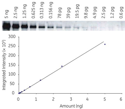
**Fig 6.10.** Fluorescence detection with Amersham ECL Plex gives a broad linear dynamic range, making it possible to detect and compare weak and strong bands on the same blot. This is a dilution series of transferrin detected with Cy3-labeled secondary antibodies. The dynamic range is 3.6 orders of magnitude and very linear with an LOD of 1.2 pg.
