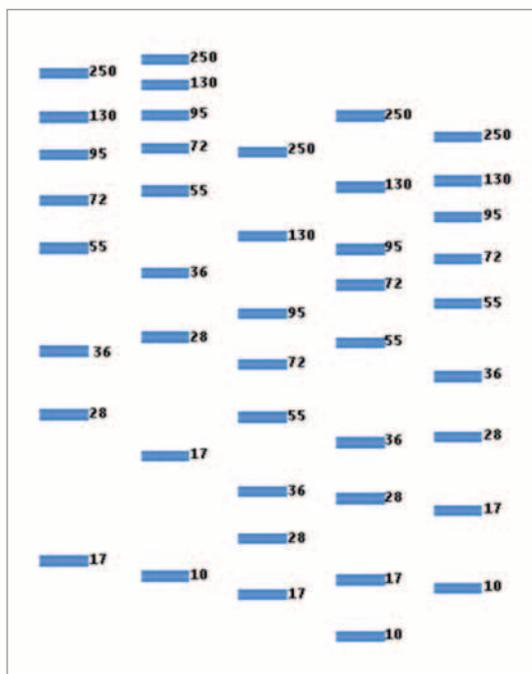
**Fig 3.3.** When selecting a gel, it is important to use an acrylamide concentration that will allow optimal separation of the proteins in your sample. High molecular weight proteins will be optimally resolved in gels containing a lower acrylamide content, while smaller proteins should ideally be run in more acrylamide-dense gels. The image shows the separation pattern for nine different proteins for each acrylamide concentration.
