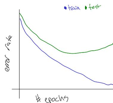
Figure 3.3: training and test error via early stopping
