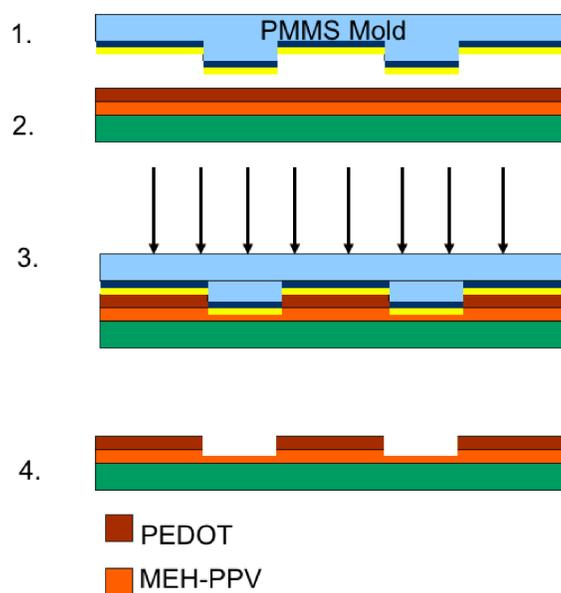
To make a 3-D cross bar circuit rotate the substrate ninety degrees every time before adding a new layer and follow the same procedures
