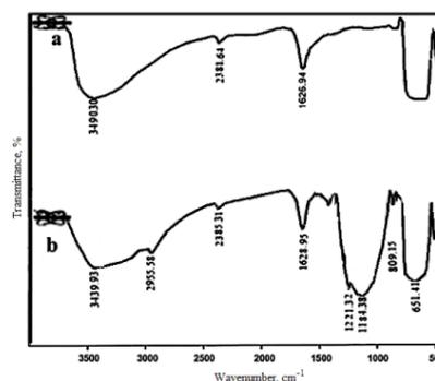
Figure 2. FT-IR spectra of (a) magnetic nanoparticles  $\text{Fe}_3\text{O}_4$ , (b) MNPs-MSA
