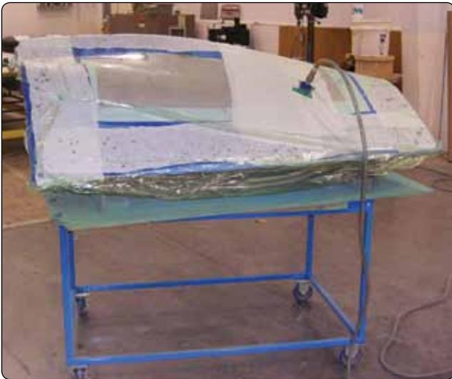
**Figure 7-52.** *Envelope bagging of repair.*
