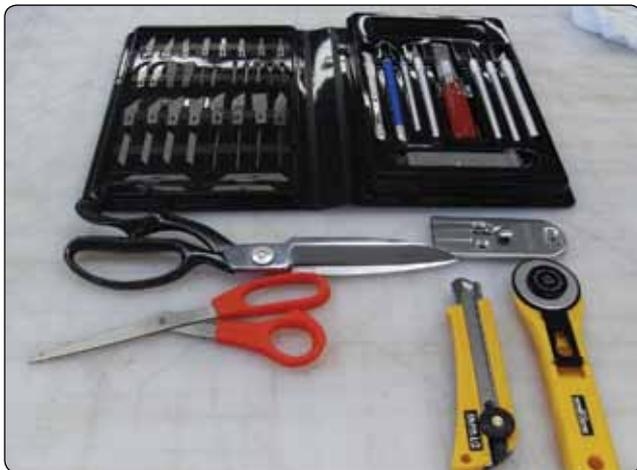
Figure 7-31. Hand tools for laminating.
