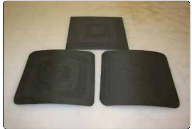
Figure 7-73. Precured patches.
