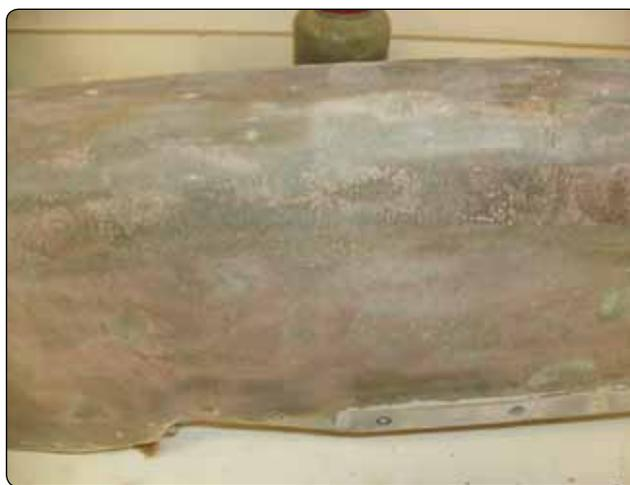
**Figure 7-8.** Copper mesh lightning protection material.
