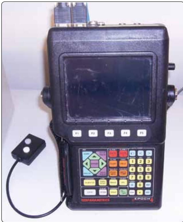
**Figure 7-26.** *Pulse echo test equipment.*
