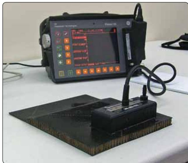
**Figure 7-28.** *Phased array testing equipment.*
