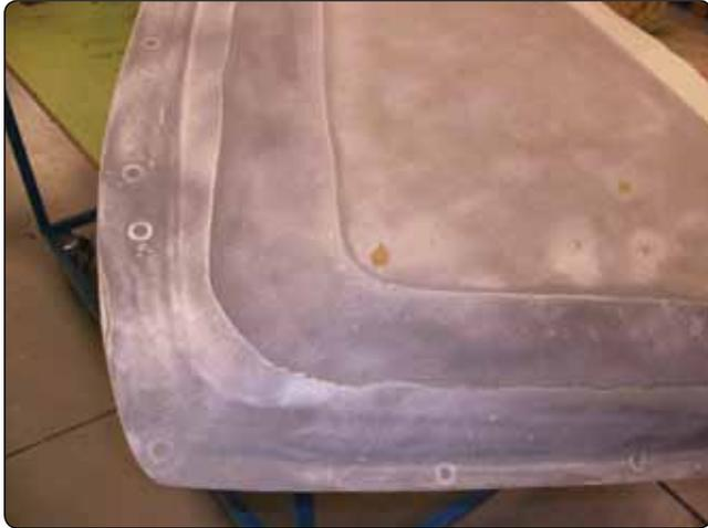
**Figure 7-9.** Aluminum mesh lightning protection material.
