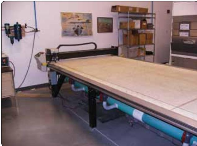
**Figure 7-89.** Gerber cutting table.
