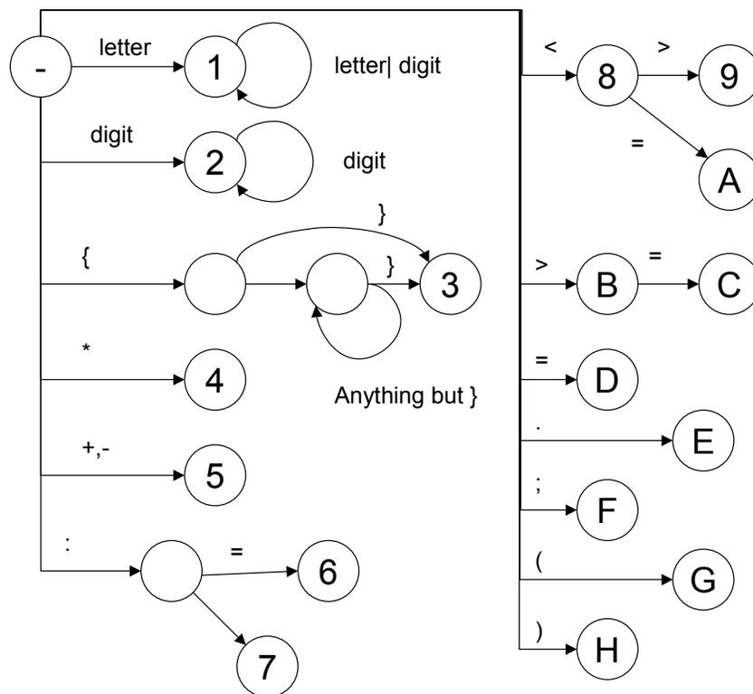
This FA handles only a subset of all Pascal tokens but it should give you an idea of how an FA can be used to drive a scanner. The numbered/lettered states are final states. The loops on states 1 and 2 continue to execute until a character other than a letter or digit is read. For example, when scanning `"temp := temp + 1;"` it would report the first token at final state 1 after reading the `"temp"` having recognized the lexeme `"temp"` as an identifier token.
