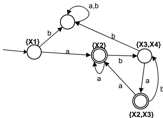
The process then goes like this: from a regular expression for a token, we construct an NFA that recognizes them using Thompson's algorithm. NFAs are not useful as drivers for programs because non-determinism implies choices and thus, expensive exhaustive backtracking algorithms. So, we use subset construction to convert that NFA to a DFA. Once we have the DFA, we can use it as the basis for an efficient non-backtracking scanner.
