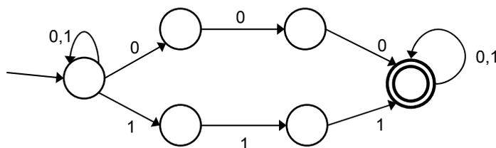
Notice that there is more than one path through the machine for a given string. For example, 000 can take you to a final state, or it can leave you in the start state. This is where the non-determinism (choice) comes in. If any of the possible paths for a string leads to a final state, that string is in the language of this automaton.
