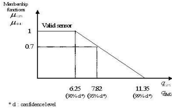
Fig. 4. Implementation of fuzzy logic to determine membership functions  $\mu_{GPS}$  and  $\mu_{IMU}$
