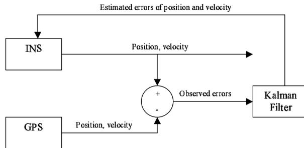
Fig. 7. Direct feedback method filter
