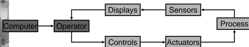
(a) Computer provides information and advice to operator (perhaps using a mechanical or electrical display, perhaps by reading sensors directly)
