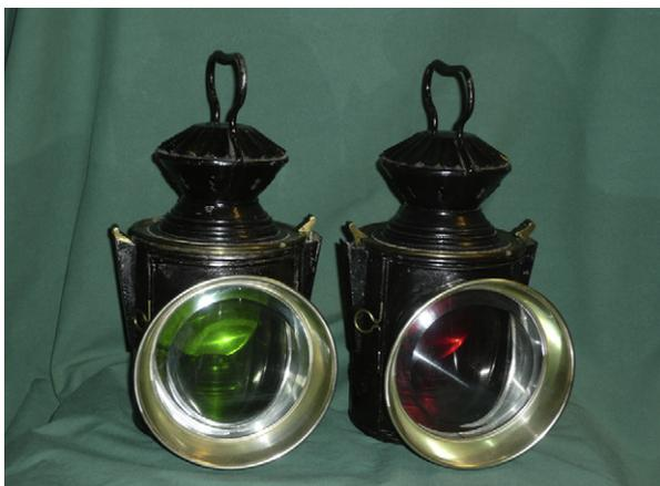
Fig. 3. Examples of railroad signal lamps from the period. By means of the handle at the top, an inner sleeve could be rotated to display red, green or clear glass. The light source was a wick, mounted above an oil reservoir and backed by a curved reflector.
